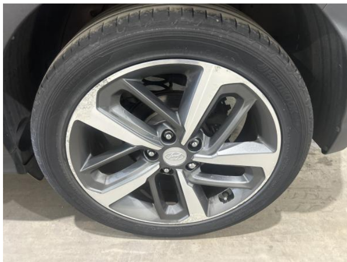
10: Wheel nsr Scratched Over 50mm
