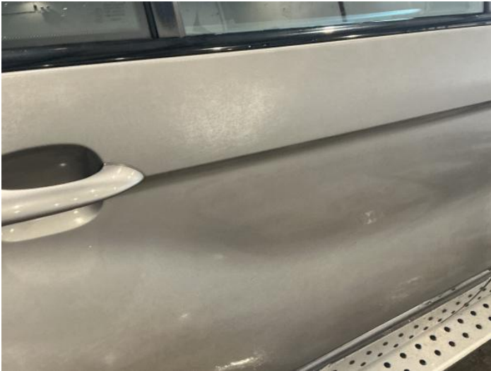
15: Door osr Poor Previous Repair Poor Paint
