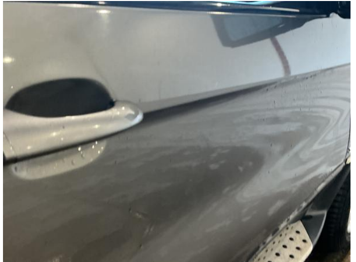
16: Door osf Poor Previous Repair Poor Paint
