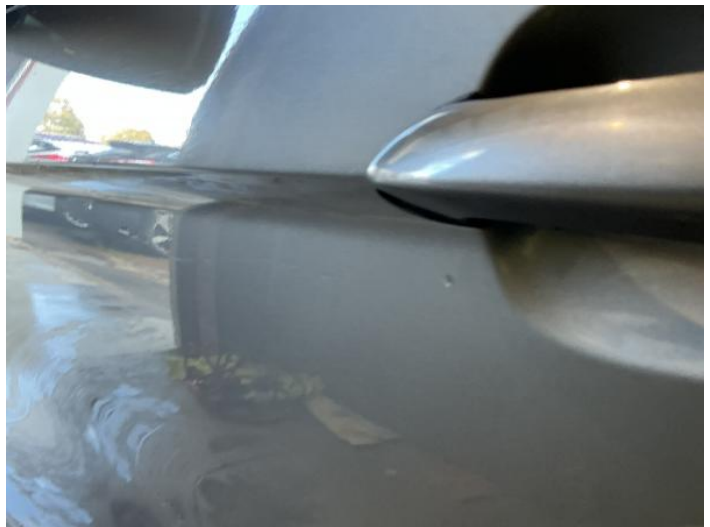
6: Door nsf Dented Over 2 UpTo 10mm
