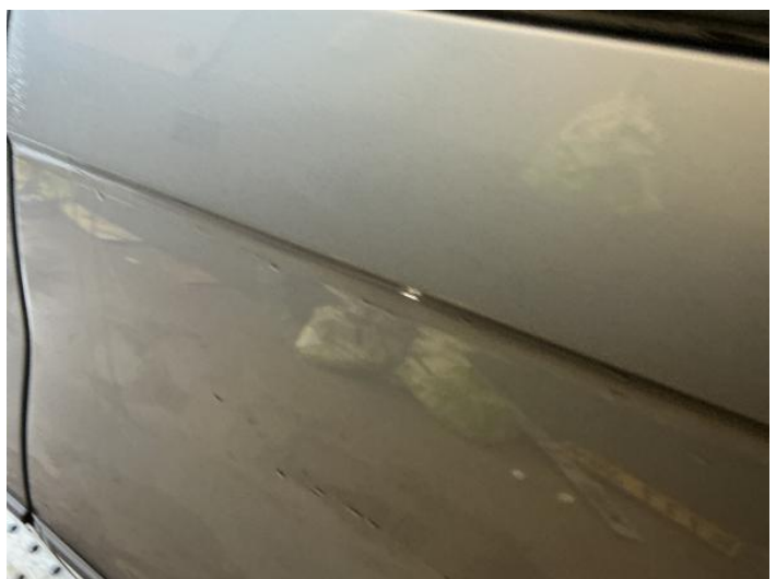
8: Door nsr Dented Over 30mm
