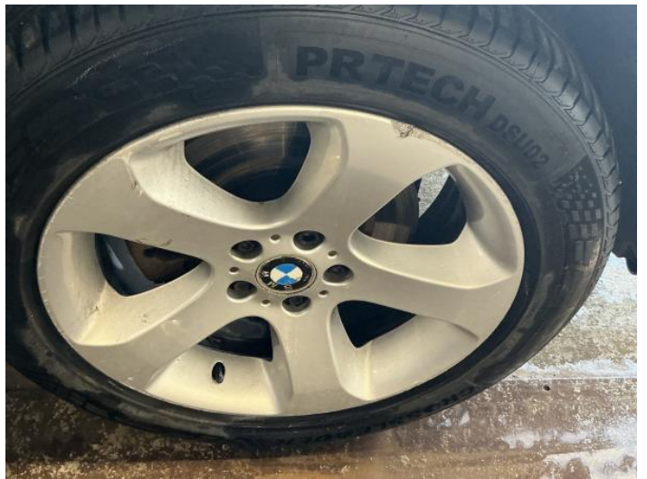
18: Wheel osf Scratched Over 50mm
