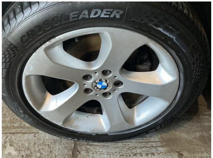
4: Wheel nsf Scratched Over 50mm
