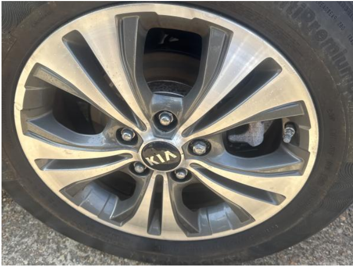
8: Wheel nsr Scratched Over 50mm
