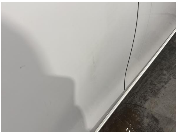
9: Door osr Scratched Over 25mm Thru Paint
