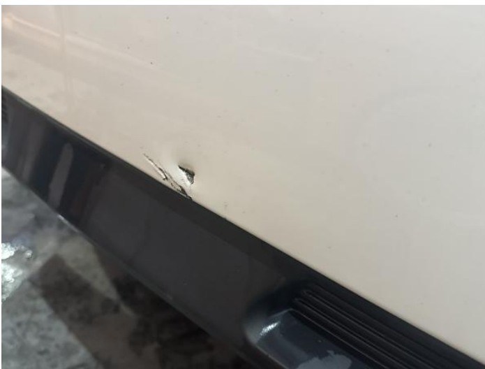
7: Bumper Rear Cracked UpTo 25mm
