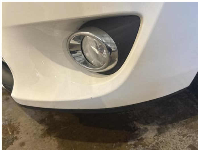
2: Bumper Front Scratched UpTo 25mm Thru Paint
