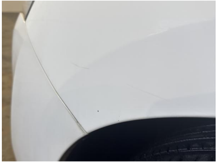
4: Wing nsf Scratched UpTo 25mm Thru Paint
