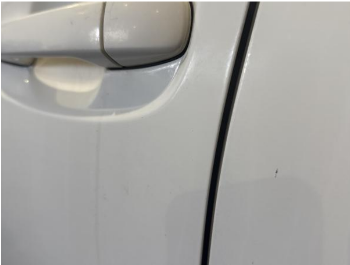
5: Door nsf Scratched UpTo 25mm Thru Paint
