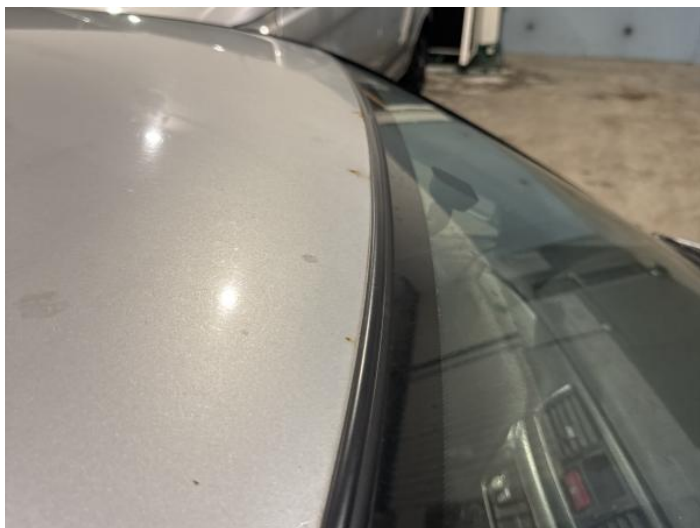
1: Roof Rusted Over 5mm
