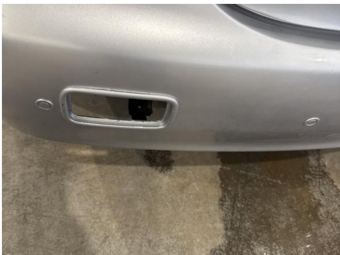
11: Reflector nsr Missing Replace
