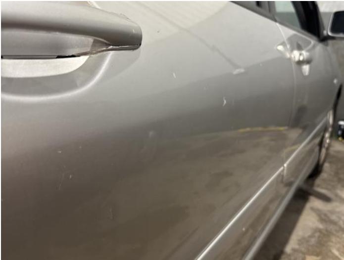
15: Door osr Dented With Paint Damage
