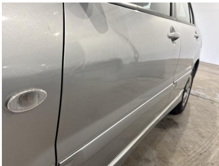
6: Door nsf Dented Over 30mm
