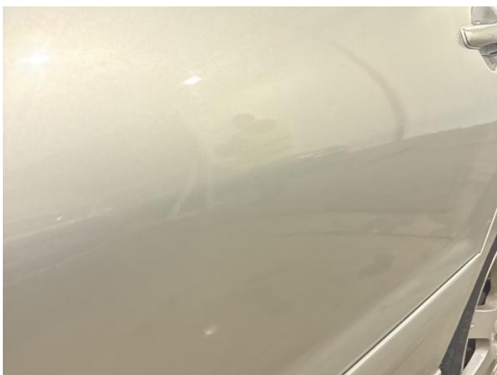
7: Door nsr Poor Previous Repair Poor Paint
