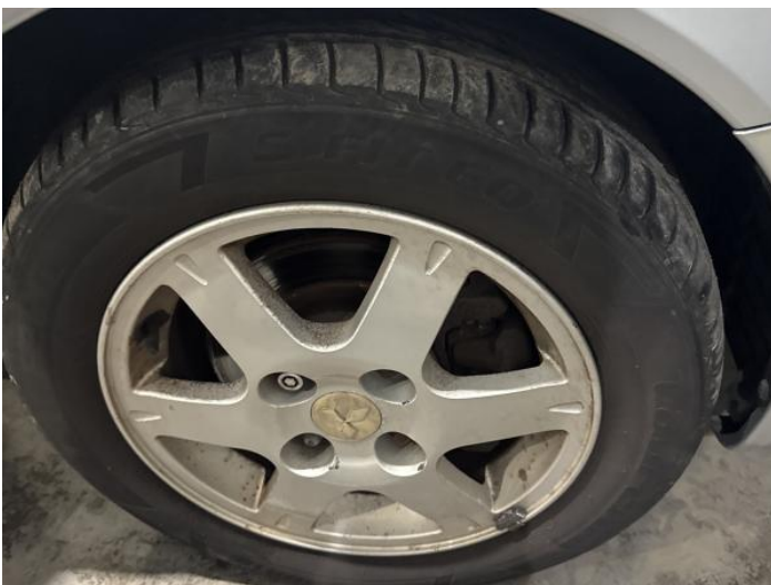
19: Wheel osf Scratched Over 50mm
