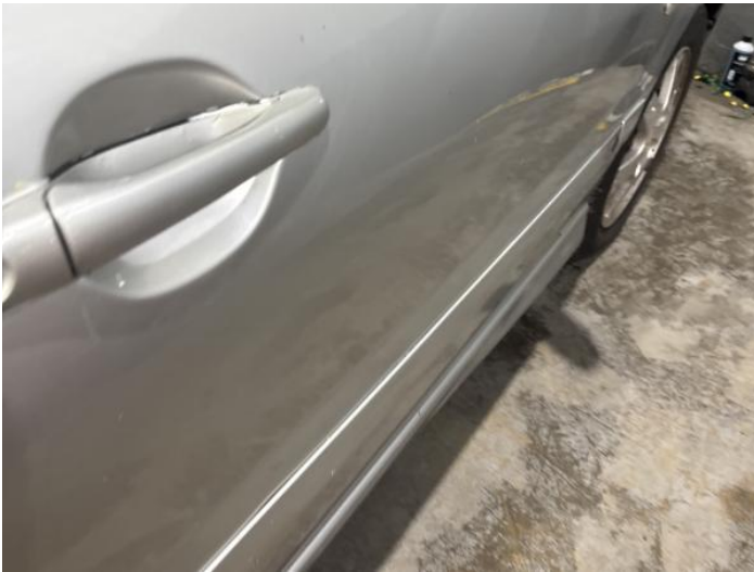
17: Door osf Dented With Paint Damage
