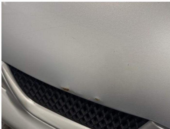
2: Bonnet Dented With Paint Damage
