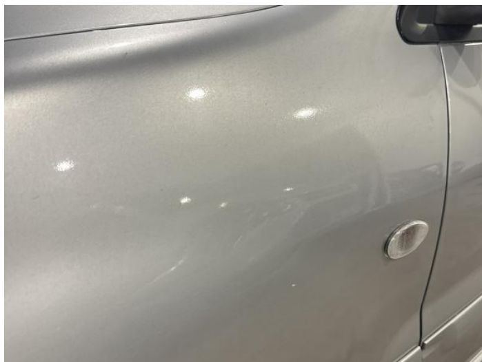
4: Wing nsf Poor Previous Repair Poor Paint
