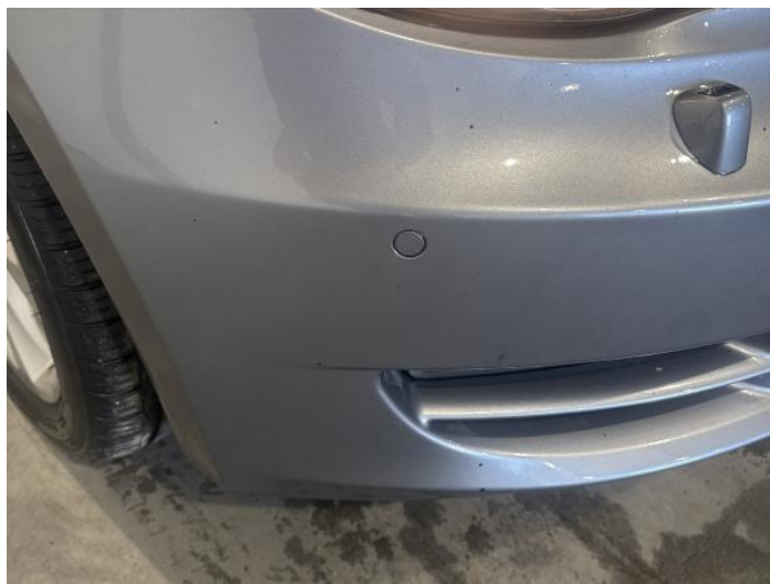
2: Bumper Front Scratched 25 to 100mm Thru Paint
