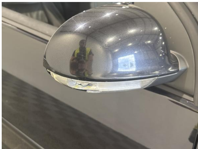
16: Flasher Side Repeater os Broken Replace
