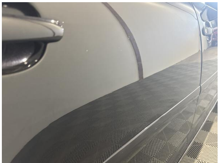
14: Door osr Dented With Paint Damage
