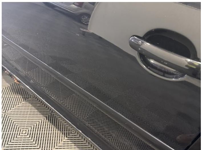
8: Door nsf Dented With Paint Damage
