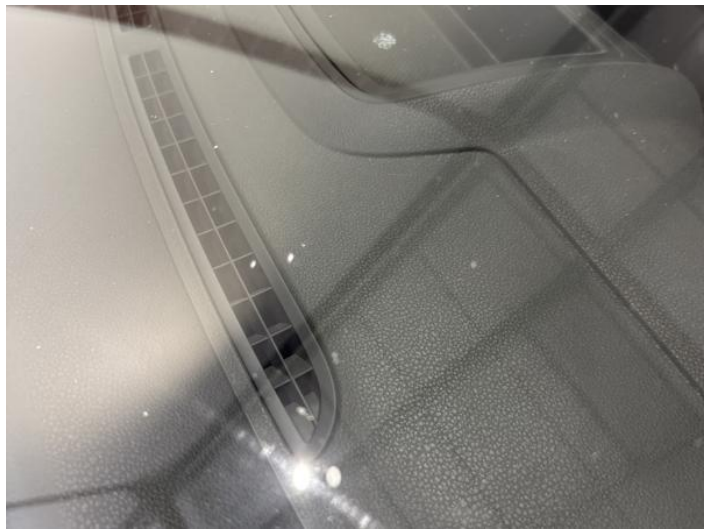
6: Screen Front Chipped Over 10mm
