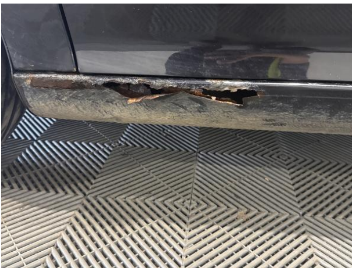
7: Sill ns Rusted Holed
