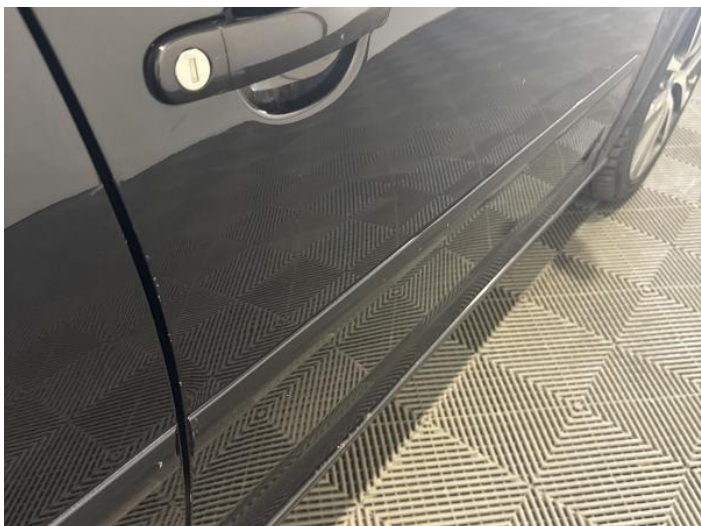
15: Door osf Dented Over 30mm
