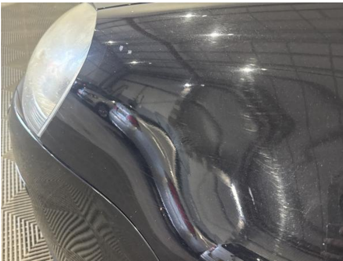
5: Wing nsf Chipped Multiple Chips
