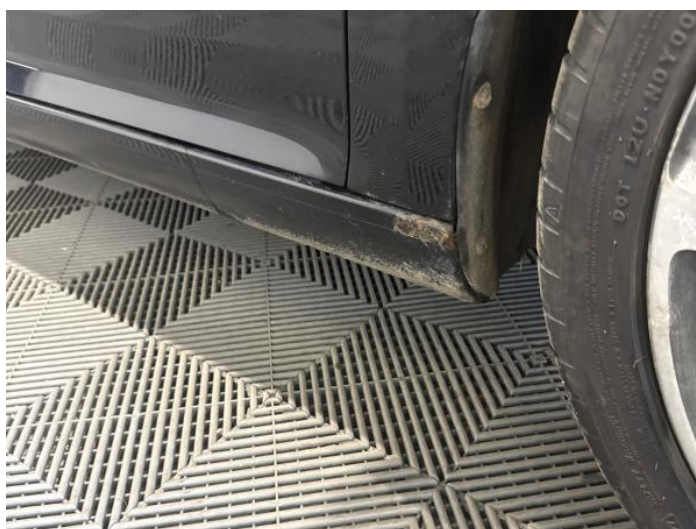
18: Sill os Rusted Over 5mm
