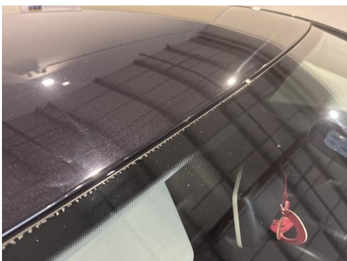
19: Roof Chipped Edge Chip
