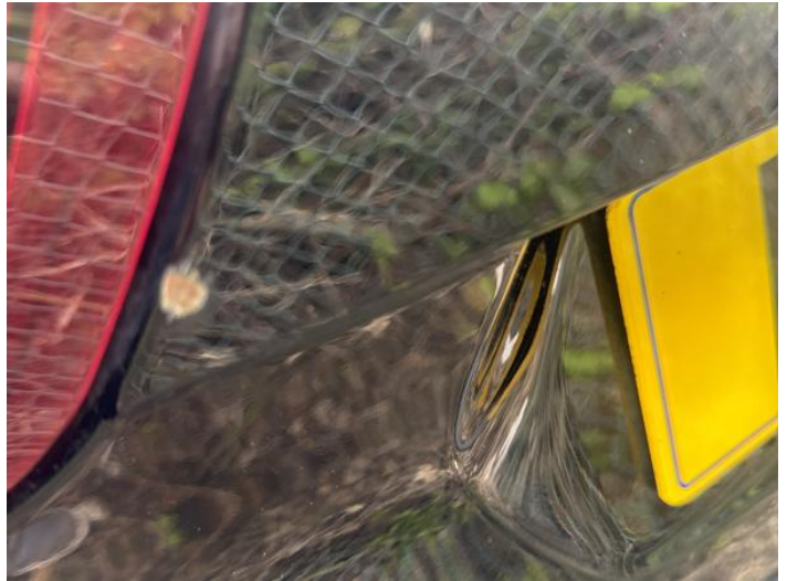
10: Boot Lid Rusted Over 5mm
