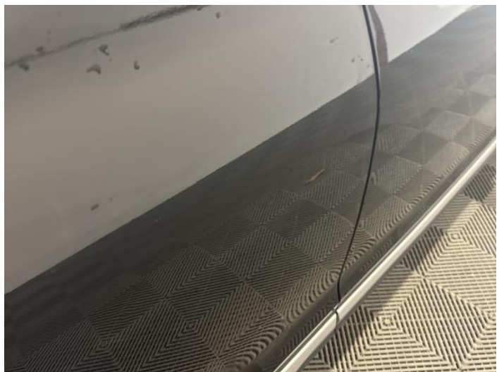
14: Door osr Dented Over 30mm
