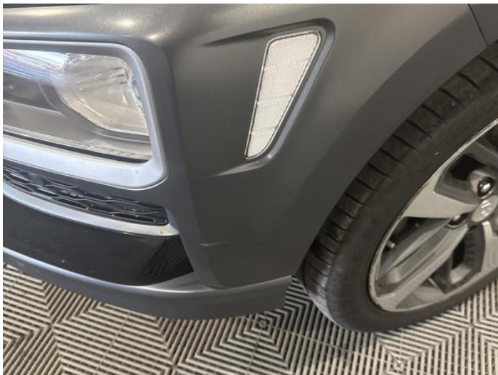
3: Bumper Front Moulding Scuffed (Unpainted) UpTo 100mm
