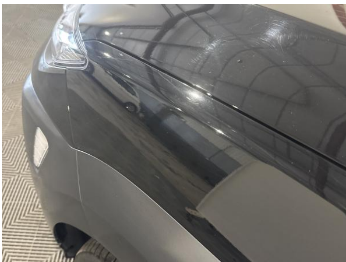
5: Wing nsf Scratched Over 25mm Thru Paint
