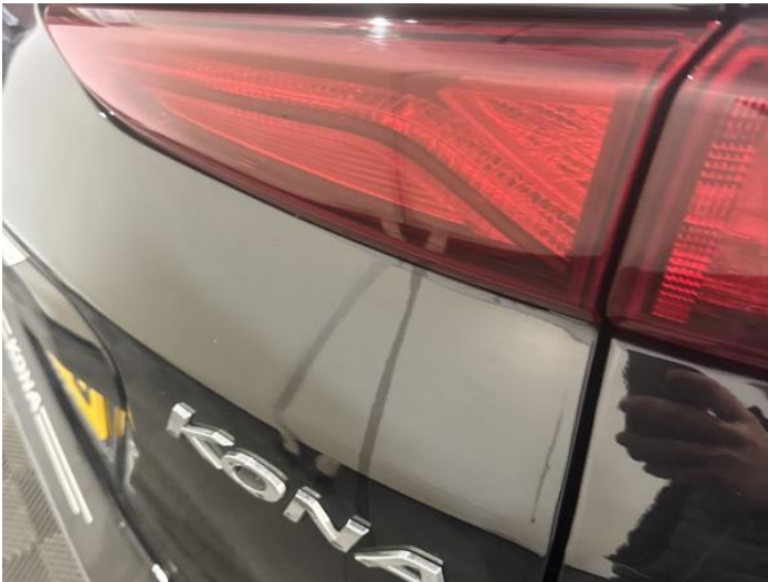
11: Tailgate Dented Between 10mm + 30mm
