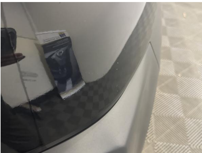
13: Qtr Panel osr Dented Between 10mm + 30mm
