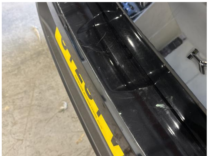
8: Bumper Rear Scratched 25 to 100mm Thru Paint
