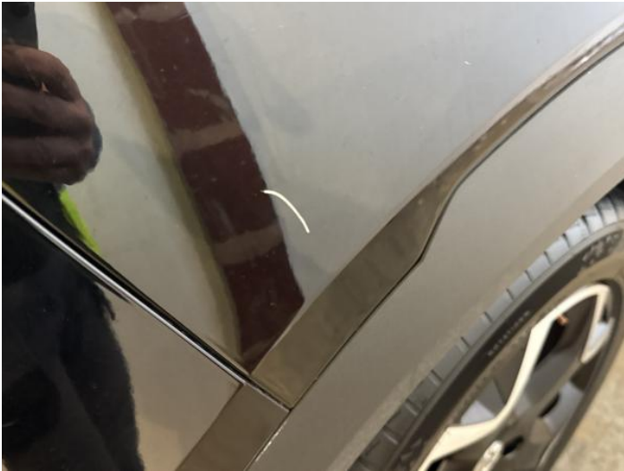
9: Qtr Panel osr Dented With Paint Damage
