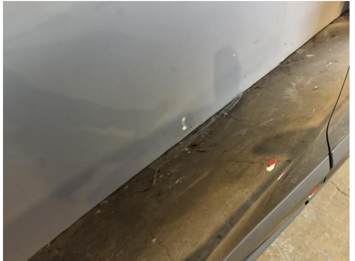
10: Door osr Scratched UpTo 25mm Thru Paint
