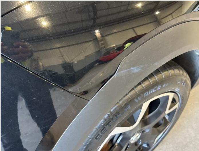
3: Wing nsf Dented Over 30mm
