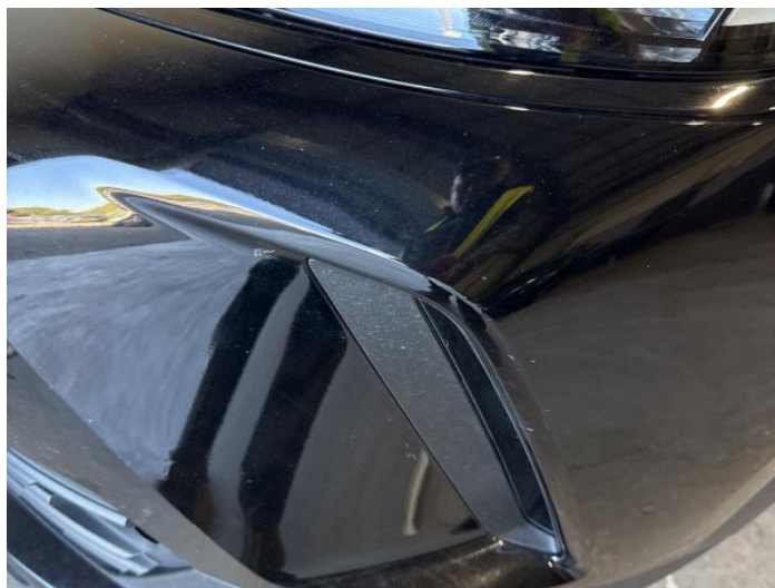
2: Bumper Front Scratched 25 to 100mm Thru Paint
