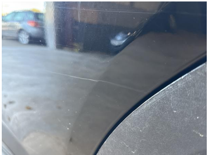
6: Door nsr Scratched Over 25mm Thru Paint
