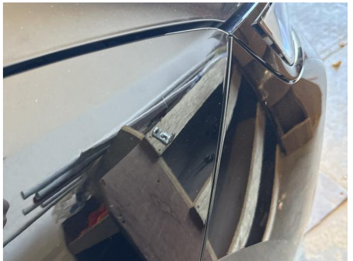
12: Wing osf Scratched UpTo 25mm Thru Paint
