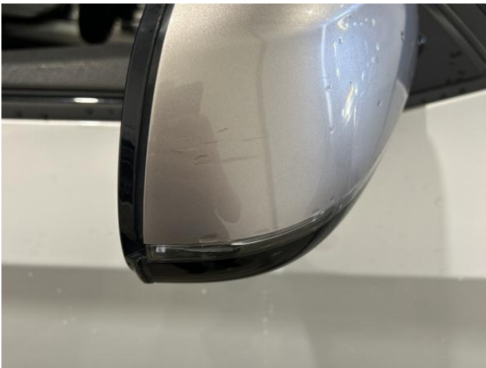
1: Door Mirror Assy osf Scratched (Painted) UpTo 25mm Not Thru Paint
