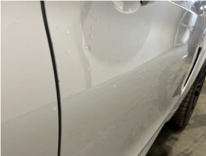
3: Door osf Dented Over 2 UpTo 10mm
