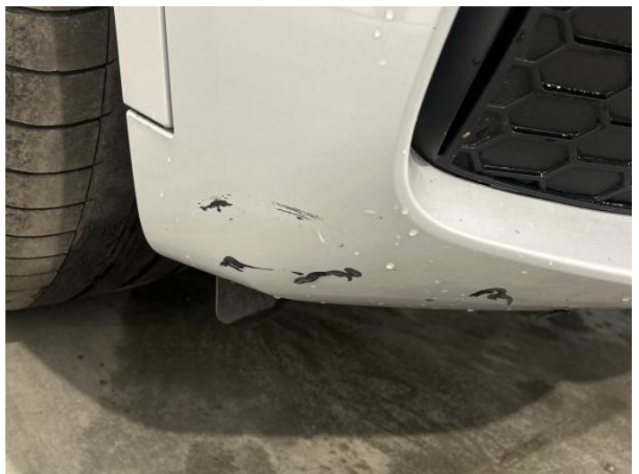
8: Bumper Front Scratched 25 to 100mm Thru Paint
