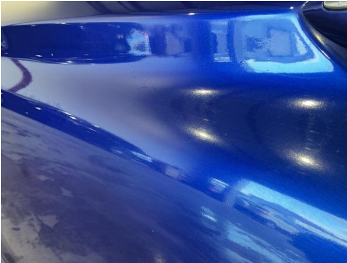
9: Door nsr Poor Previous Repair Poor Paint
