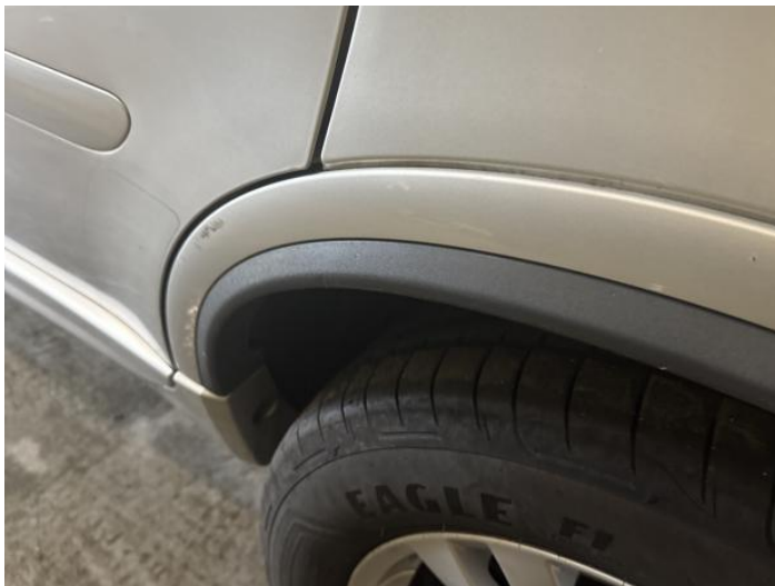
9: Qtr Panel Arch Extension ns Scratched (Painted) Over 25mm Thru Paint
