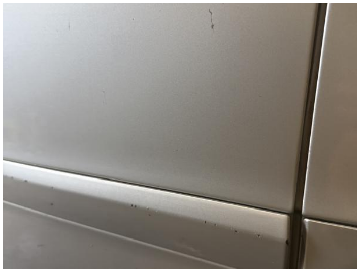
6: Door nsf Scratched UpTo 25mm Thru Paint
