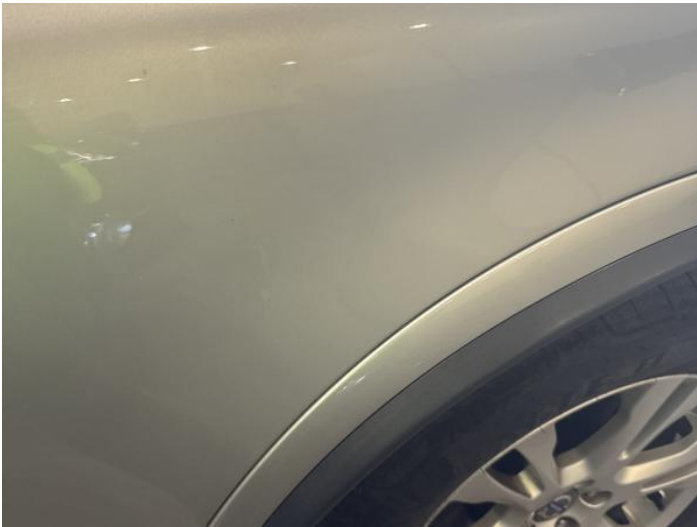
17: Wing osf Scratched Over 25mm Thru Paint
