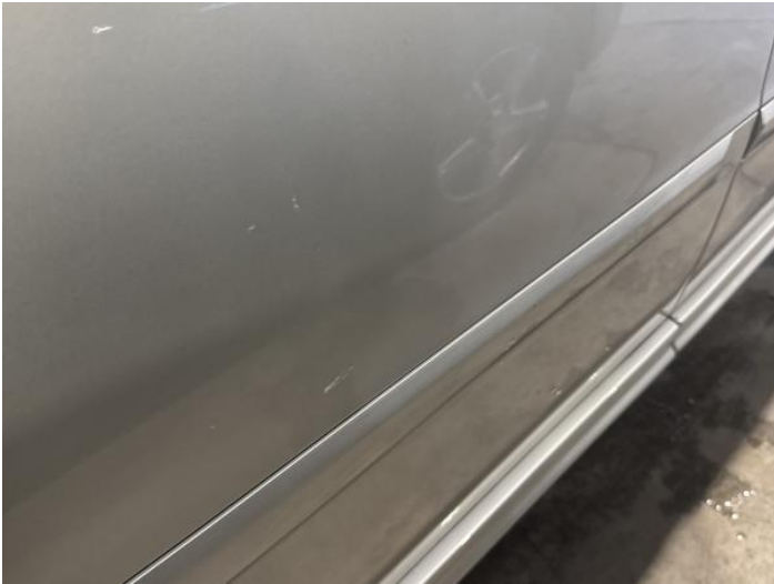
15: Door osr Scratched Over 25mm Thru Paint
