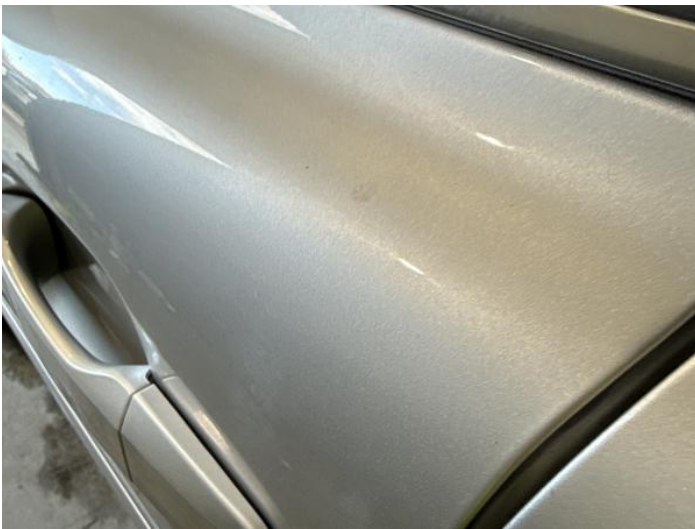
5: Door nsf Dented Between 10mm + 30mm
