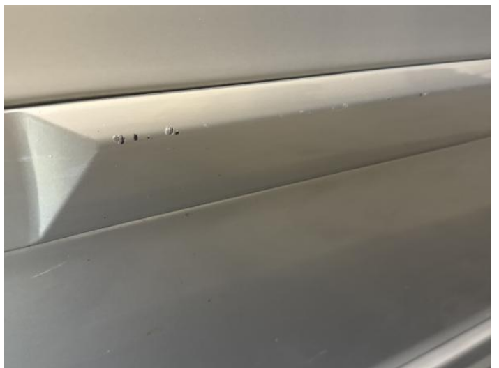
8: Door Moulding nsr Scratched (Painted) Over 25mm Thru Paint
