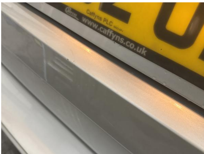
11: Tailgate Scratched UpTo 25mm Thru Paint
