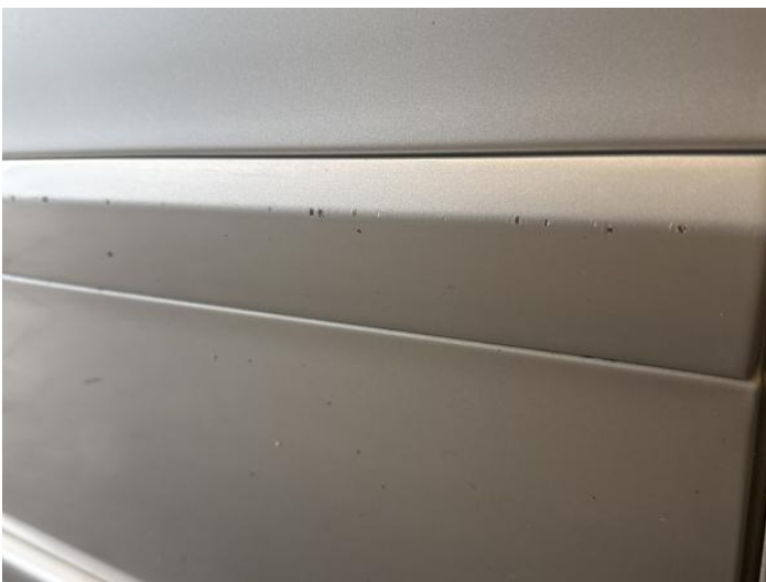
7: Door Moulding nsf Scratched (Painted) Over 25mm Thru Paint
