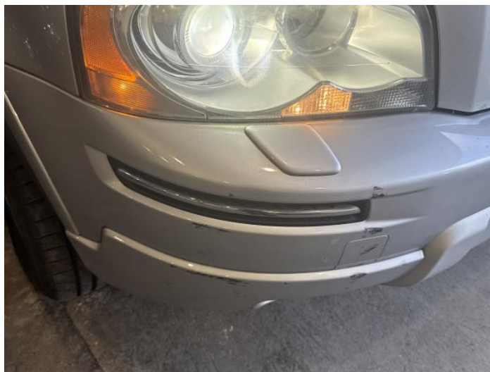
2: Bumper Front Scratched 25 to 100mm Thru Paint
