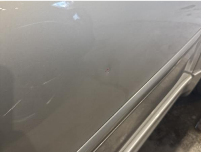
16: Door osf Dented 2 Or Less UpTo 10mm
