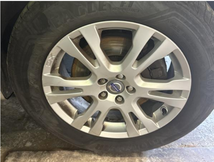
18: Wheel osf Scratched Over 50mm
