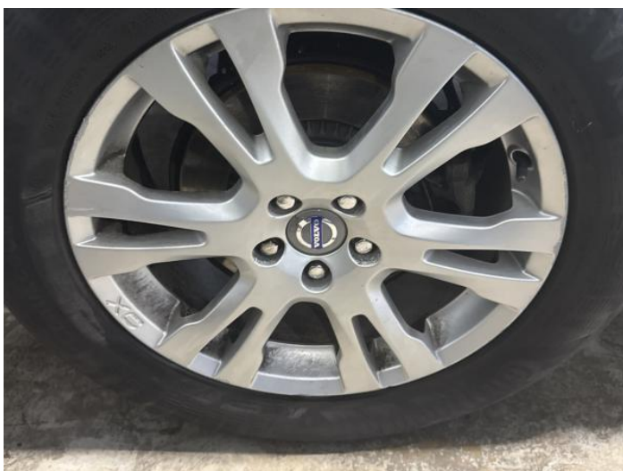
13: Wheel osr Scratched Over 50mm
