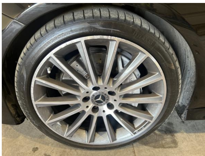
6: Wheel nsf Scratched Over 50mm
