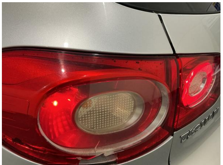
14: Lamp nsr Broken Replace
