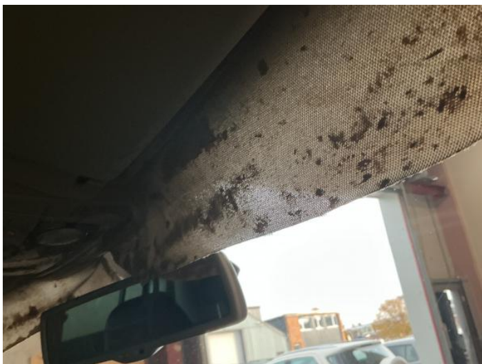
1: Roof Lining Torn Over 3mm
