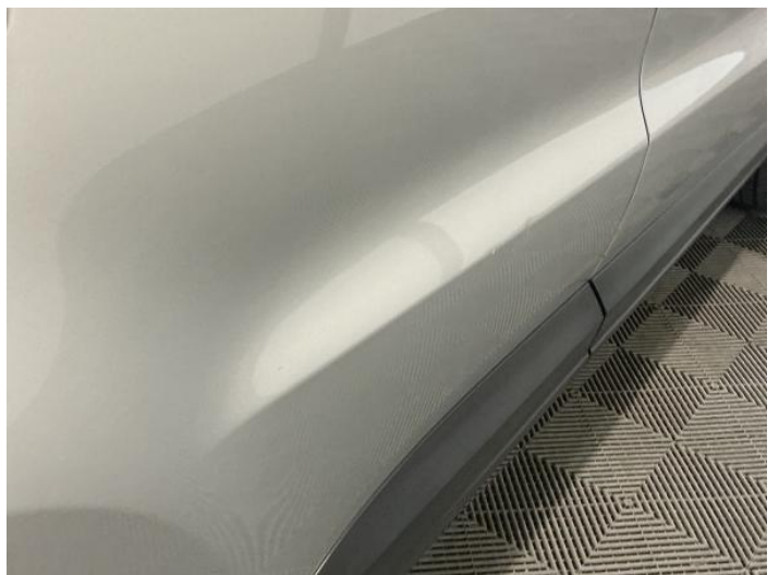
20: Door osr Dented With Paint Damage
