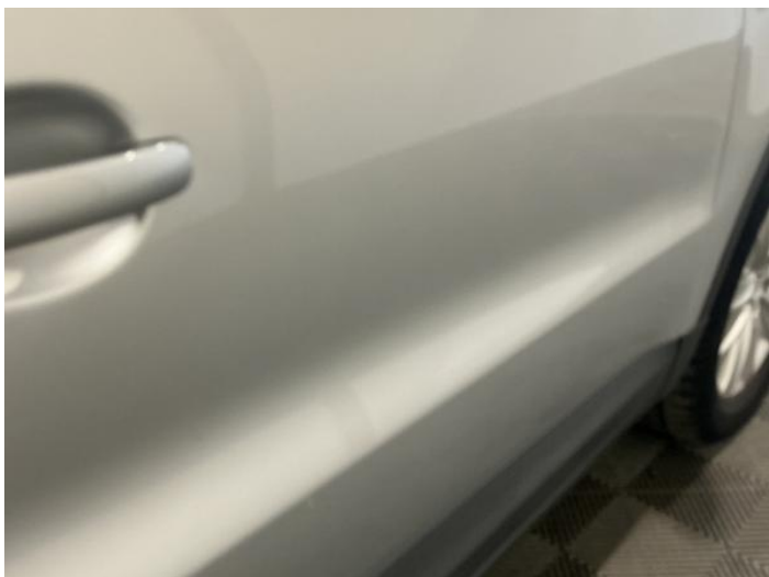
21: Door osf Dented With Paint Damage
