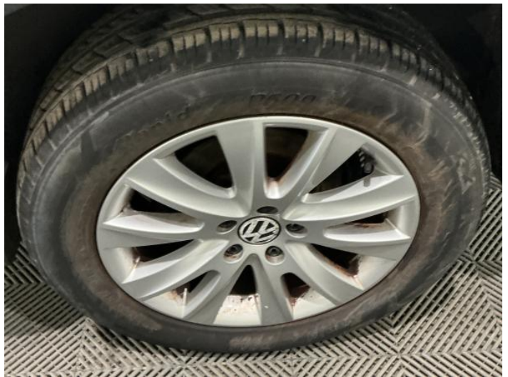
12: Wheel nsr Scratched Up To 50mm
