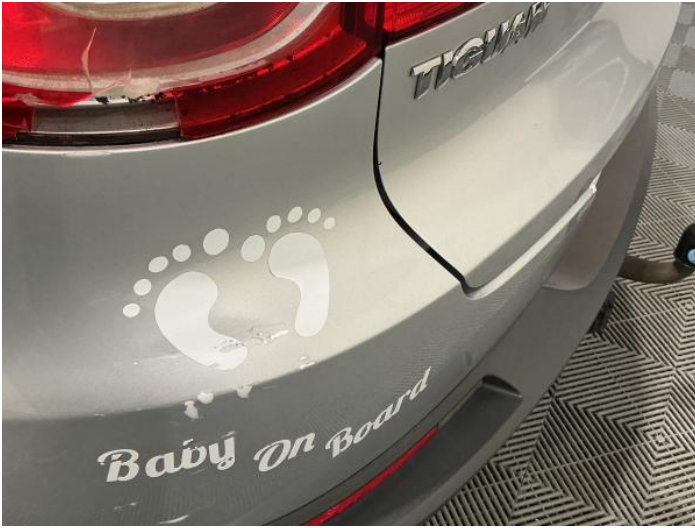
15: Bumper Rear Dented With Paint Damage
