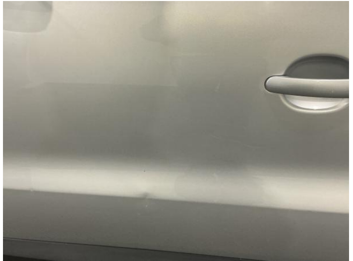
10: Door nsf Dented With Paint Damage
