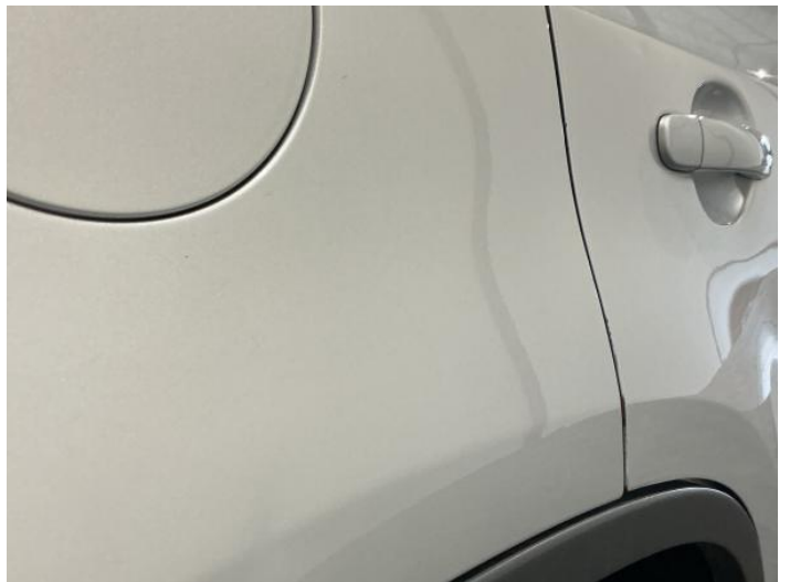
18: Qtr Panel osr Dented Over 30mm
