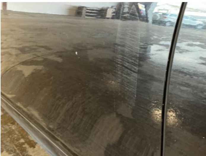
7: Door nsf Dented With Paint Damage
