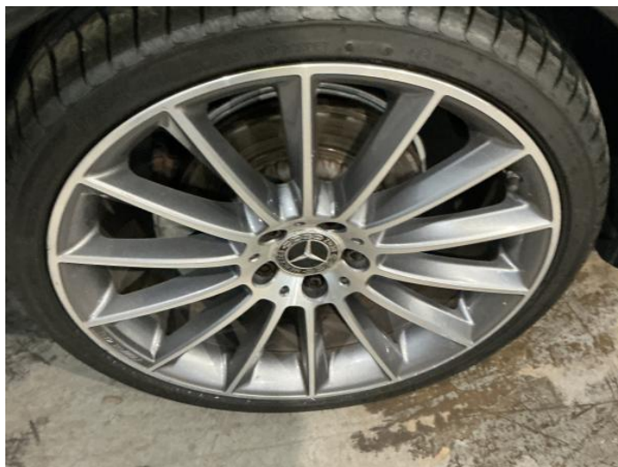
16: Wheel osr Scratched Over 50mm
