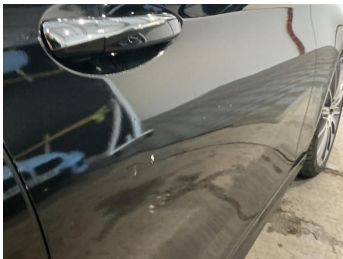
18: Door osf Dented With Paint Damage
