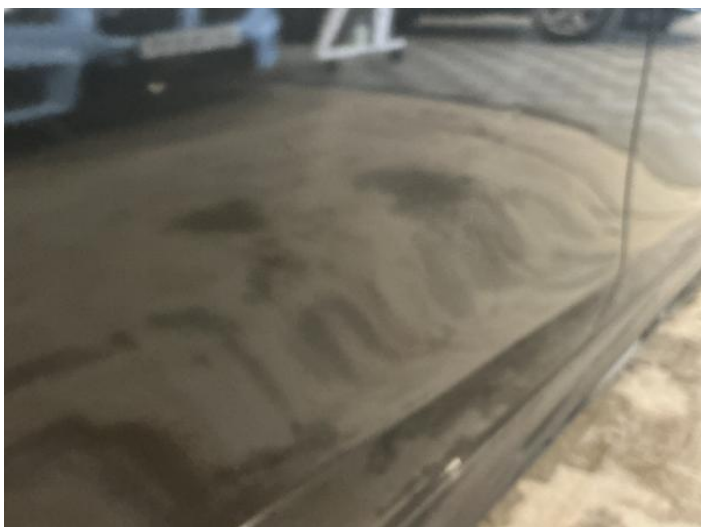
17: Door osr Poor Previous Repair Poor Paint
