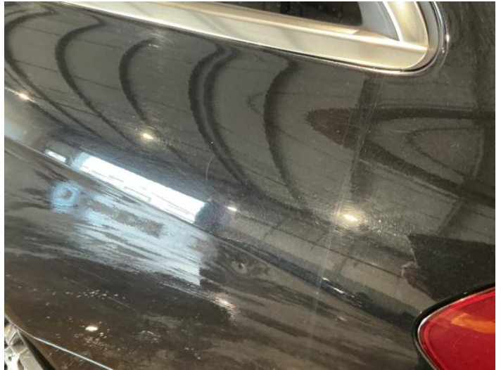
10: Qtr Panel nsr Dented Over 2 UpTo 10mm
