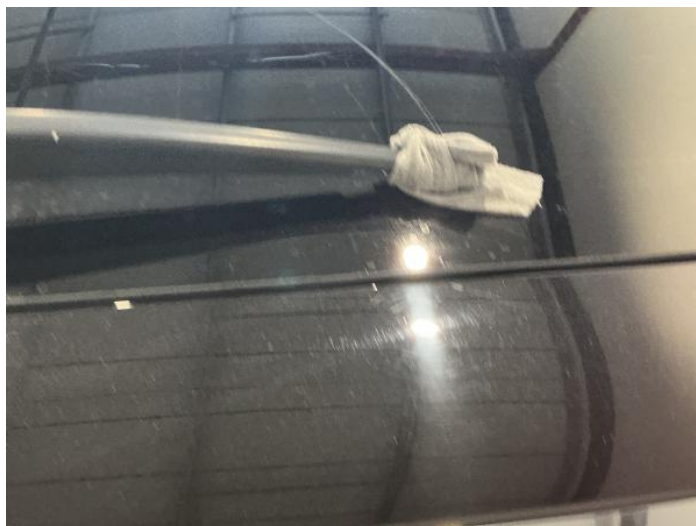
22: Wiper Rear Broken Replace
