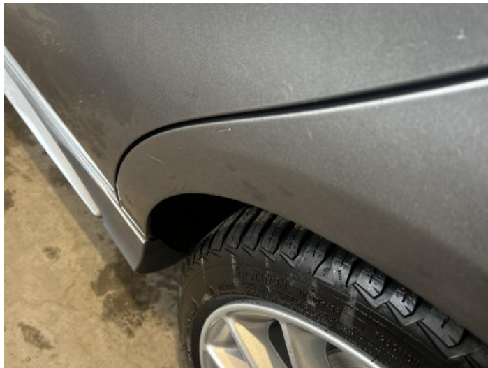
4: Qtr Panel nsr Scratched UpTo 25mm Thru Paint
