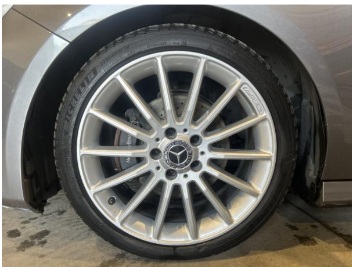
7: Wheel nsf Scratched Up To 50mm
