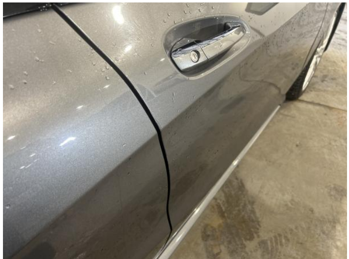
2: Door osf Chipped Edge Chip
