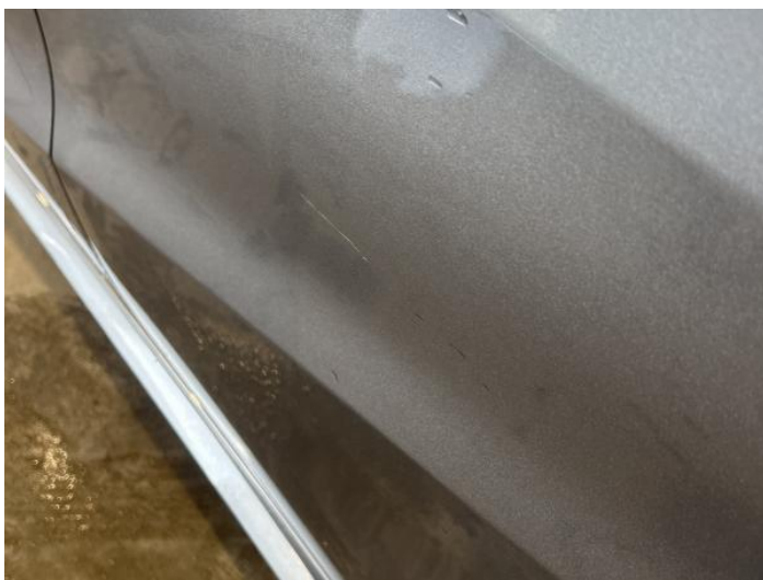
5: Door nsr Scratched Over 25mm Not Thru Paint
