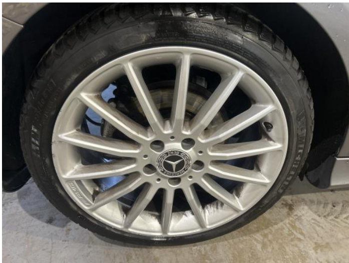
3: Wheel osr Scratched Over 50mm
