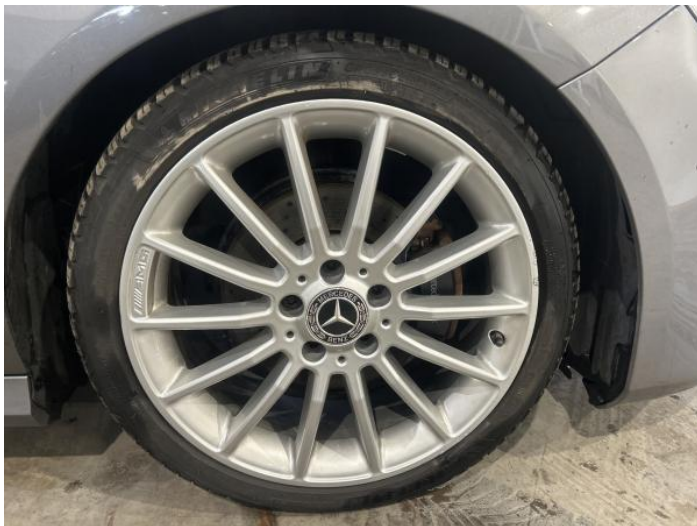
1: Wheel osf Scratched Up To 50mm
