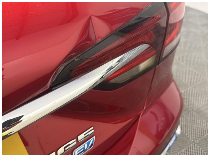
14: Lamp osr Broken Replace
