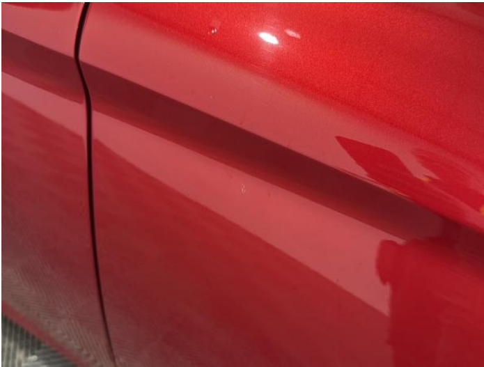
11: Wing osf Scratched Up To 25mm Thru Paint
