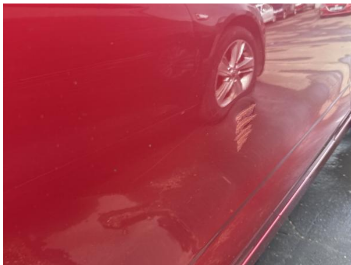
4: Door nsf Dented With Paint Damage
