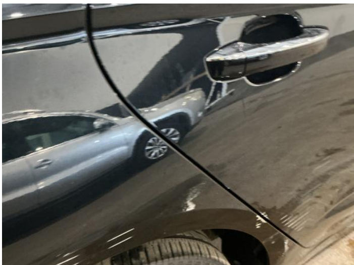
9: Qtr Panel osr Dented With Paint Damage
