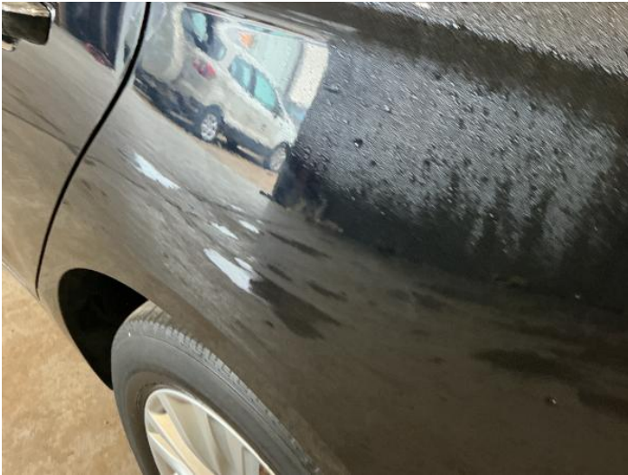
15: Qtr Panel nsr Dented Over 30mm
