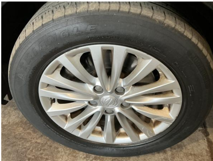
21: Wheel nsf Scratched Over 50mm
