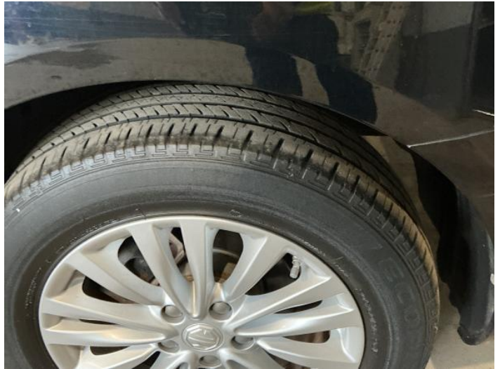
16: Wheel nsr Scratched Up To 50mm
