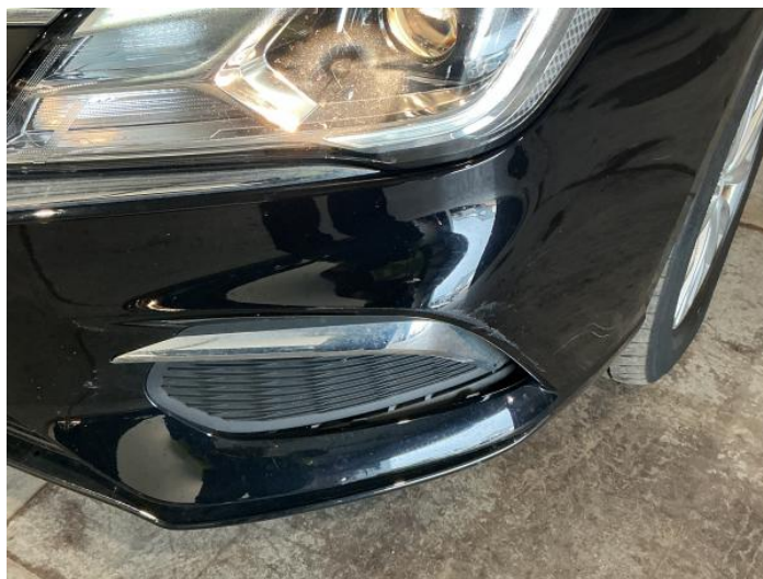
2: Fog Lamp Surrounds Broken Replace
