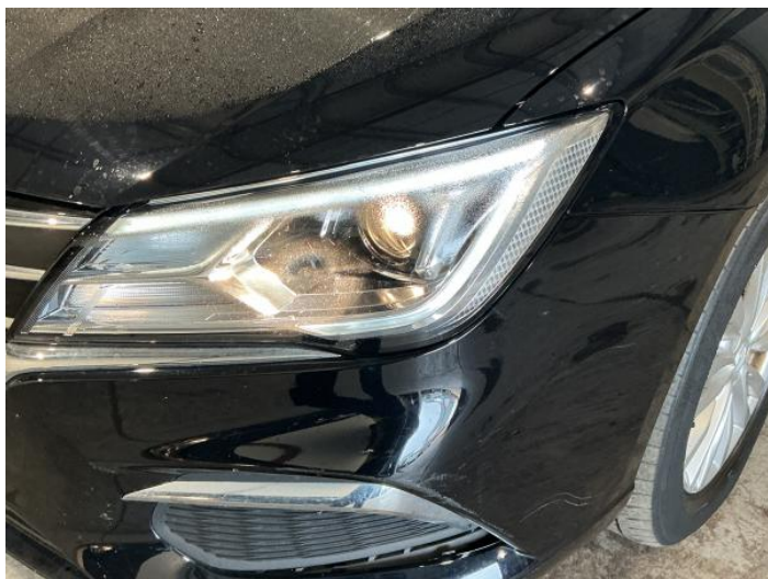
1: Bumper Front Scratched Over 100mm Thru Paint
