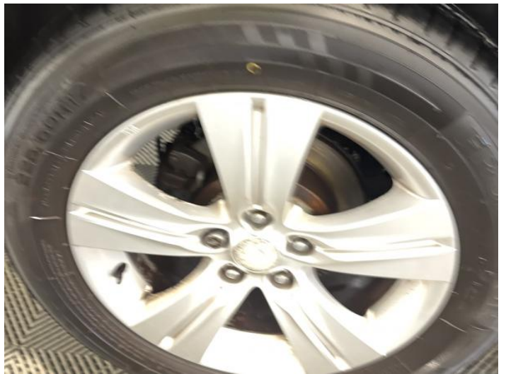
18: Wheel osr Scratched Over 50mm
