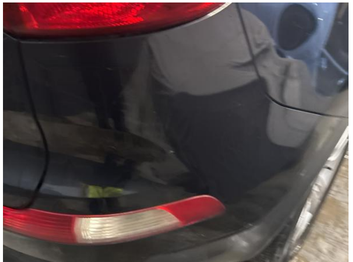
12: Bumper Rear Scratched 25 to 100mm Thru Paint
