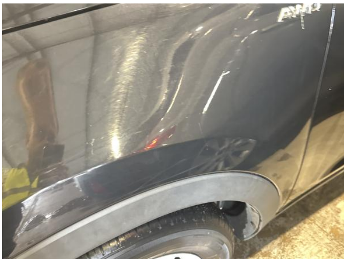
3: Wing nsf Scratched Over 25mm Thru Paint
