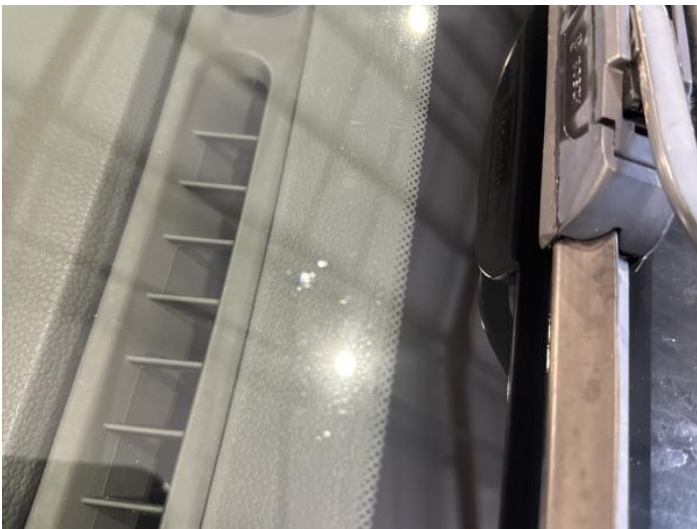
23: Screen Front Chipped UpTo 10mm
