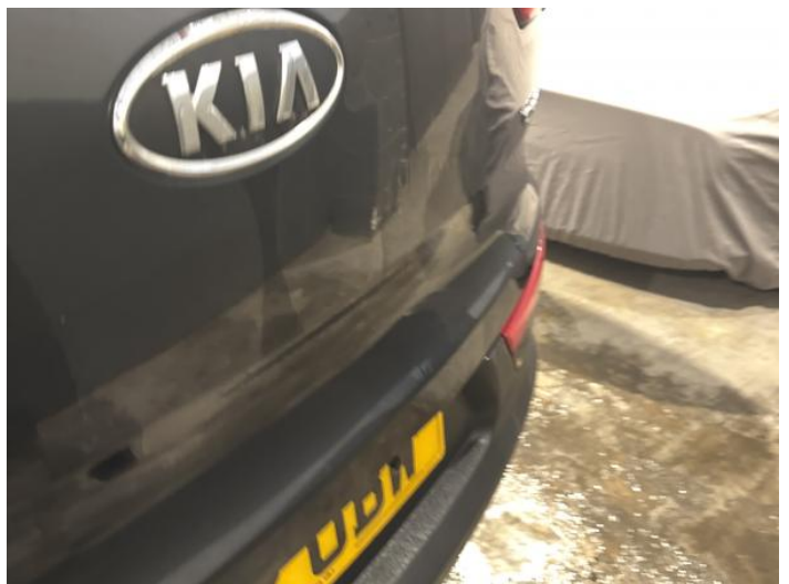
14: Boot Lid Dented Over 2 UpTo 10mm
