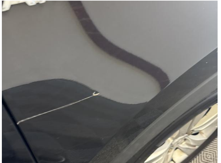
22: Wing osf Dented With Paint Damage
