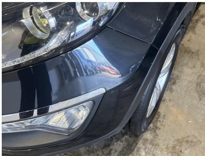
2: Bumper Front Scratched Over 100mm Thru Paint
