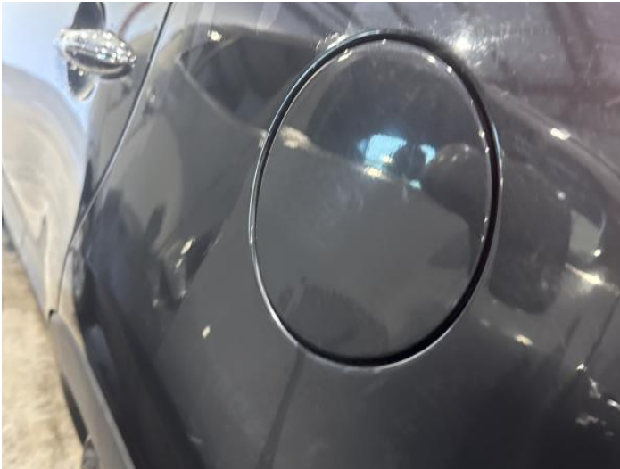
9: Qtr Panel nsr Chipped 1 To 5
