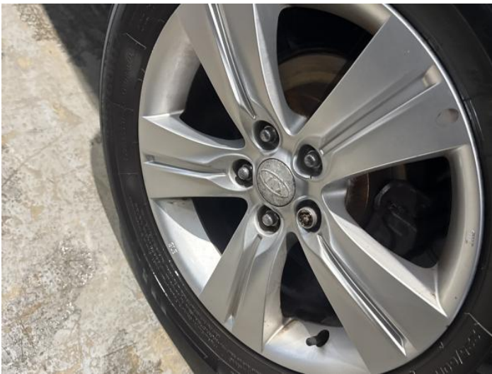
11: Wheel nsr Scratched Up To 50mm
