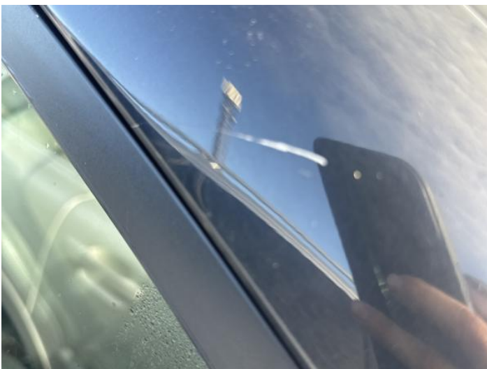
25: A Post os Scratched UpTo 25mm Thru Paint
