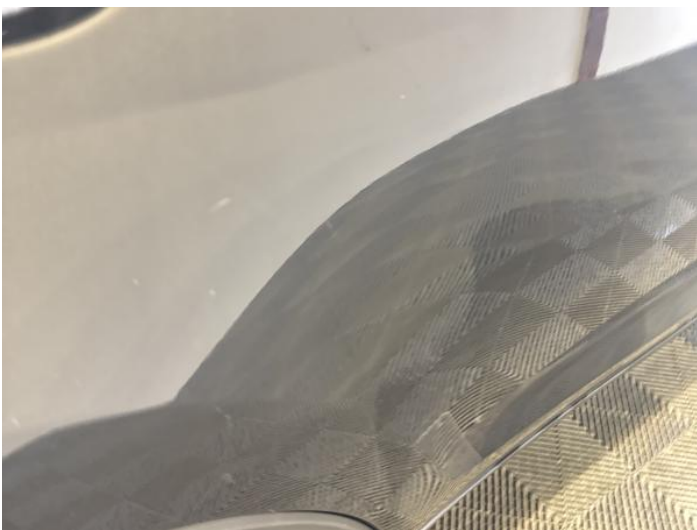
19: Door osr Dented With Paint Damage
