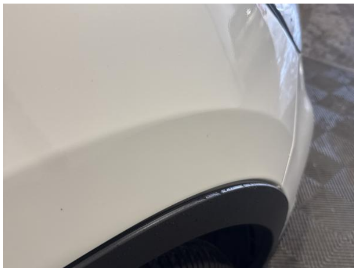
10: Wing osf Poor Previous Repair Rippled UpTo 30%
