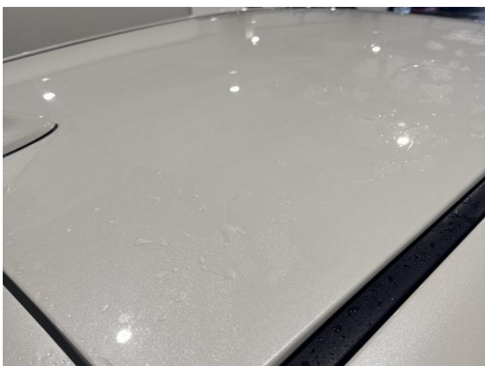
11: Roof Dented Over 30mm
