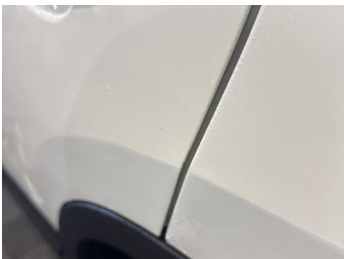
5: Door nsr Chipped Edge Chip
