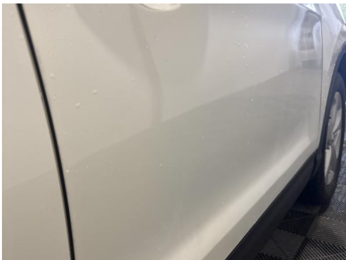
9: Door osf Poor Previous Repair Rippled UpTo 30%
