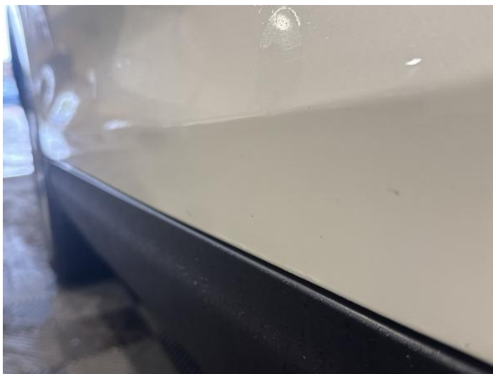
4: Door nsf Dented Over 30mm
