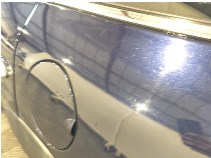
9: Qtr Panel nsr Dented Over 2 UpTo 10mm
