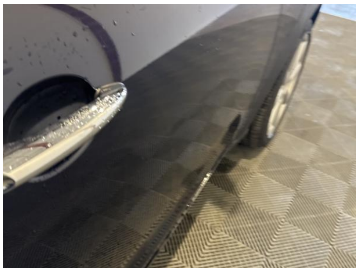
18: Door osf Dented Over 2 UpTo 10mm
