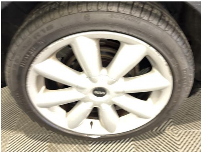
15: Wheel osr Scratched Over 50mm
