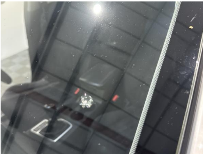
23: Screen Front Chipped Over 10mm
