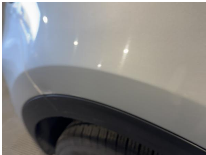
4: Wing nsf Dented With Paint Damage
