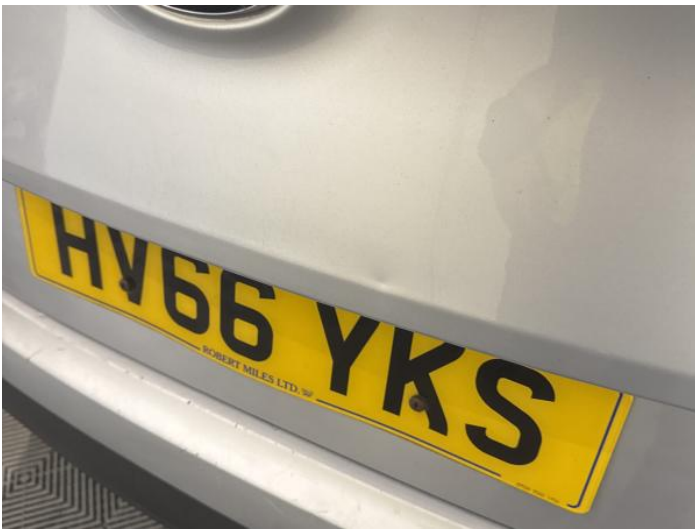
11: Boot Lid Dented Over 30mm
