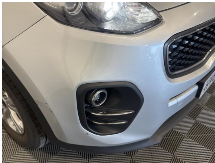
2: Bumper Front Scratched Over 100mm Thru Paint
