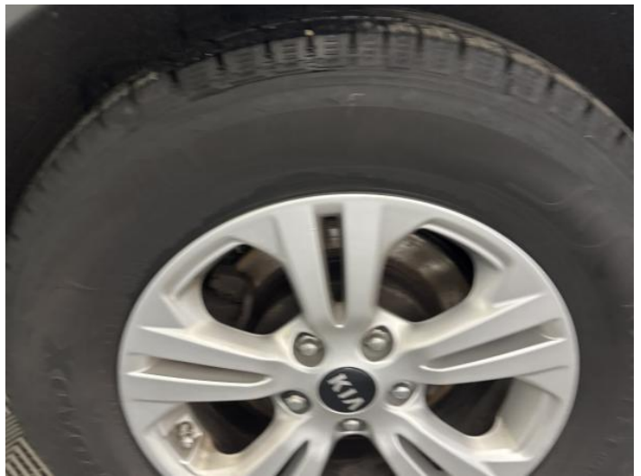
12: Wheel osr Scratched Up To 50mm
