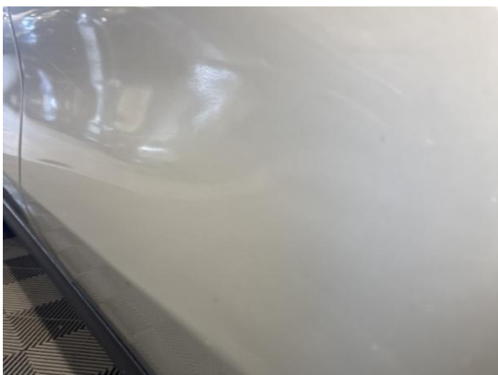
7: Door nsr Dented With Paint Damage
