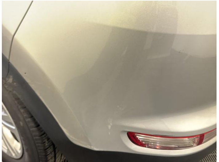
10: Bumper Rear Scratched Over 100mm Thru Paint
