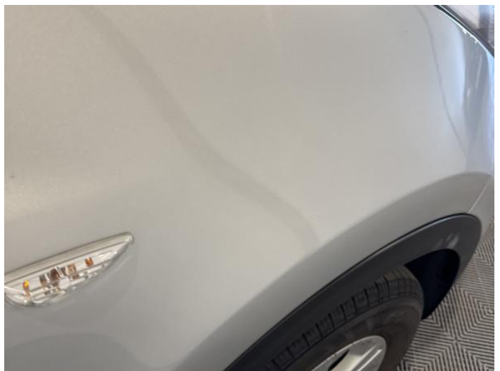
20: Wing osf Dented Over 2 UpTo 10mm
