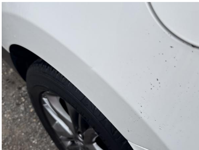
8: Qtr Panel nsr Dented Between 10mm + 30mm
