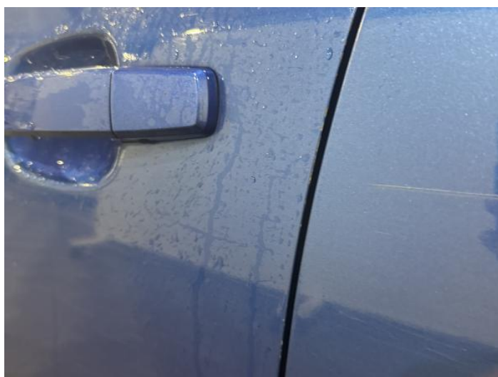
6: Door nsf Chipped Edge Chip
