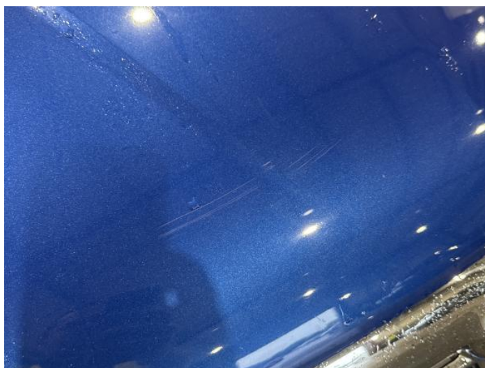
2: Bonnet Scratched Over 25mm Thru Paint
