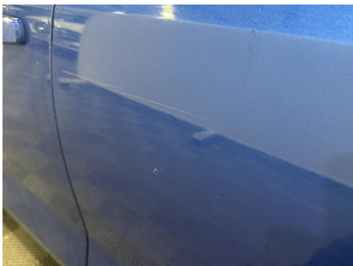
7: Door nsr Scratched Over 25mm Thru Paint
