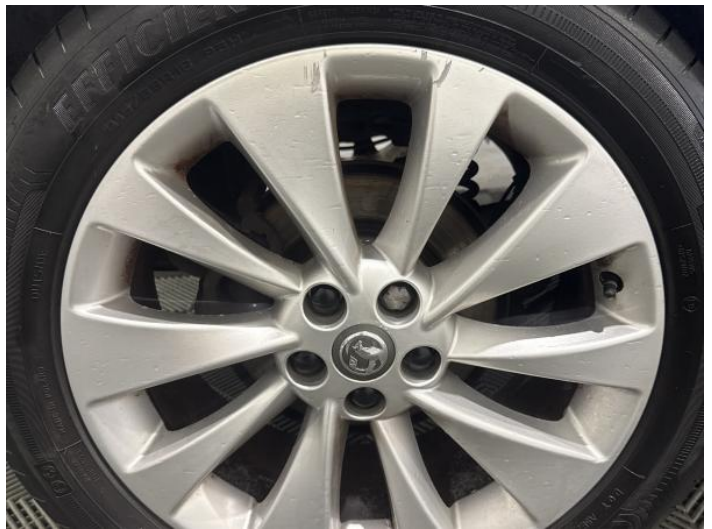
12: Wheel osr Scratched Over 50mm
