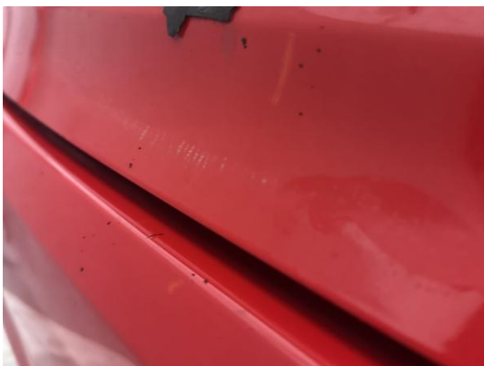
13: Boot Lid Scratched Over 25mm Thru Paint
