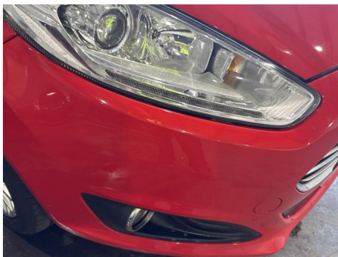
2: Bumper Front Scratched Over 100mm Thru Paint
