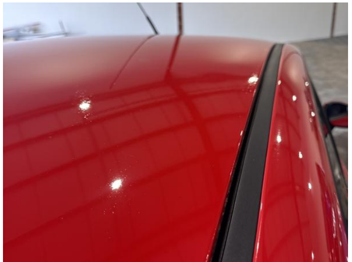
22: Roof Dented Over 30mm
