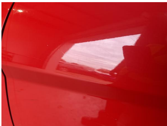
8: Door nsr Scratched Over 25mm Thru Paint
