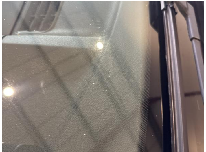
18: Screen Front Chipped UpTo 10mm
