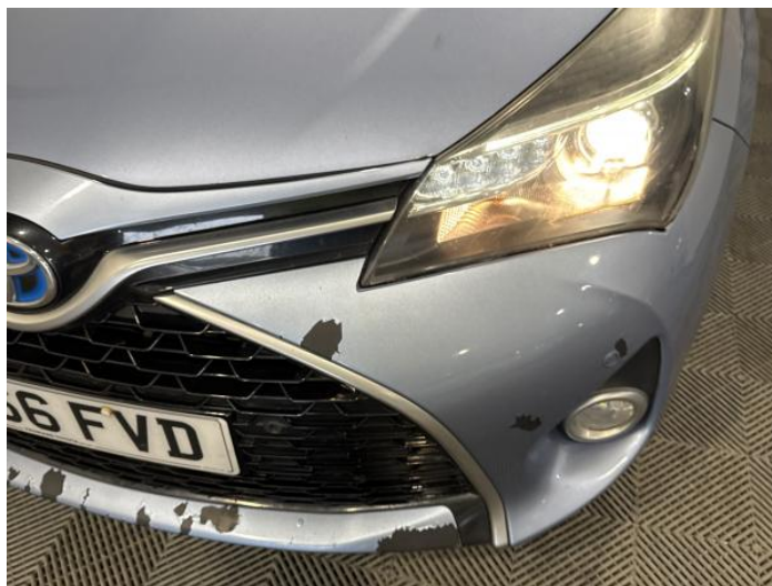
2: Bumper Front Poor Previous Repair Paint Flake
