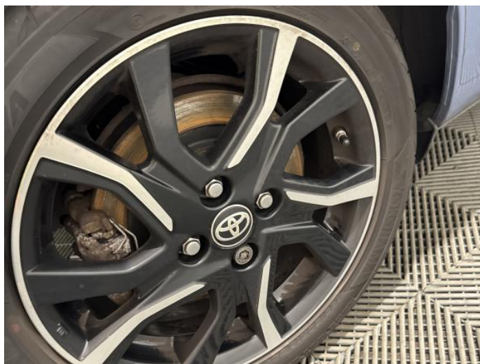
12: Wheel osr Scratched Up To 50mm
