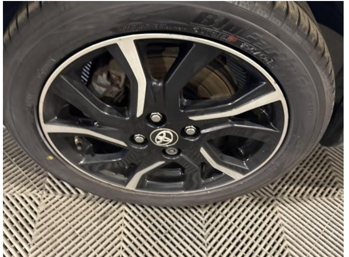
4: Wheel nsf Scratched Up To 50mm
