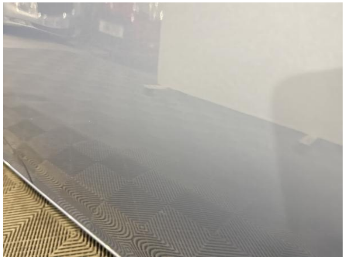
6: Door nsr Dented Between 10mm + 30mm
