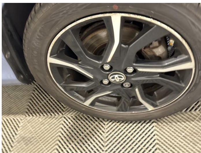
18: Wheel osf Scratched Over 50mm
