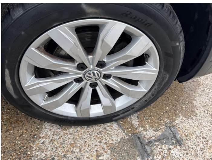
19: Wheel osf Scratched Up To 50mm
