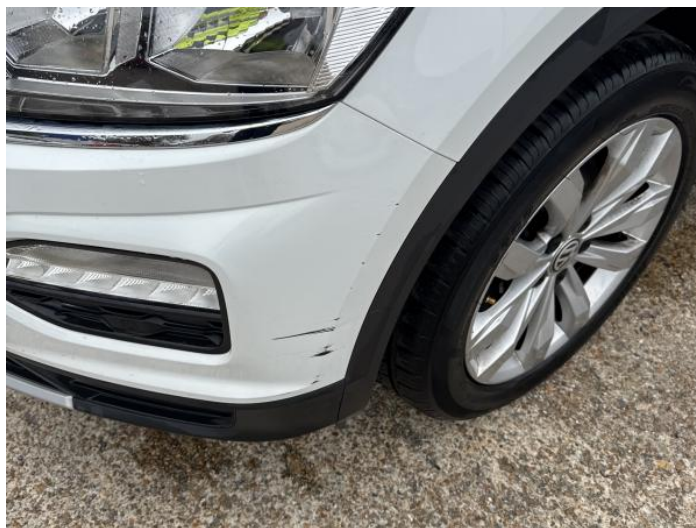
2: Bumper Front Scratched Over 100mm Thru Paint
