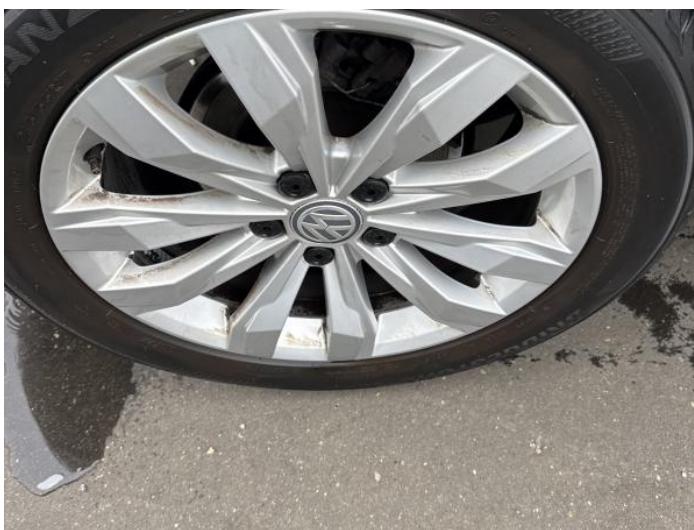
14: Wheel osr Scratched Up To 50mm
