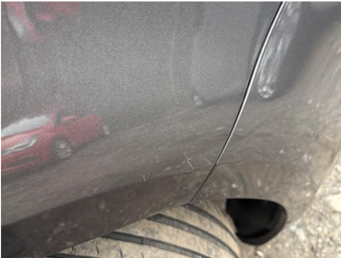
17: Wing osf Scratched UpTo 25mm Thru Paint
