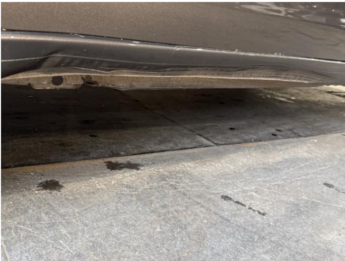
19: Sill ns Dented Over 30mm
