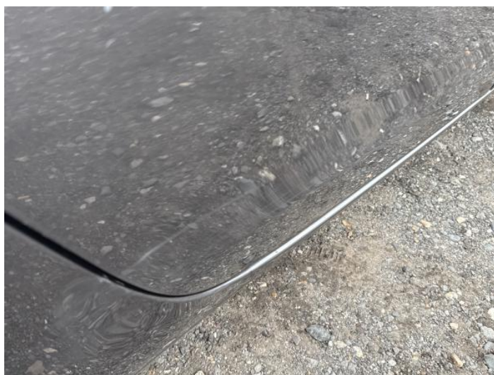
14: Door osr Scratched Over 25mm Thru Paint
