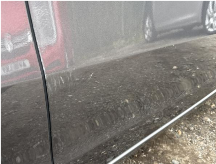
15: Door osf Scratched Over 25mm Thru Paint
