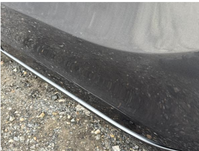
7: Door nsr Scratched Over 25mm Thru Paint
