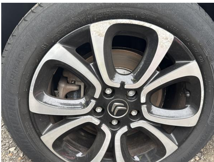
13: Wheel osr Corroded Light
