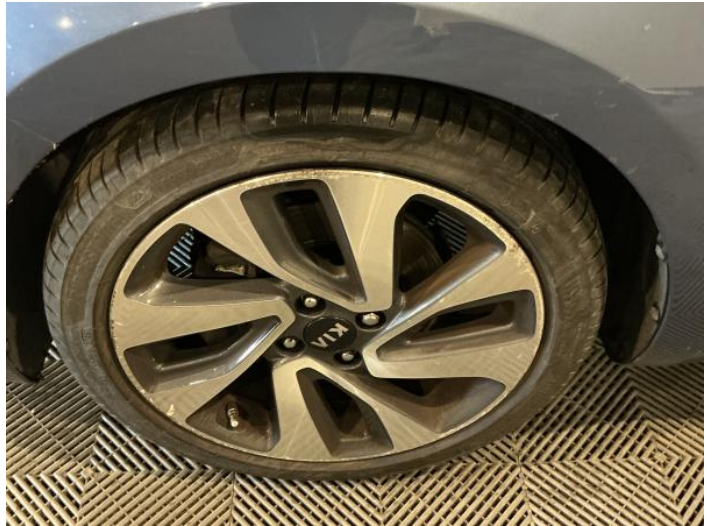
4: Wheel nsf Scratched Over 50mm
