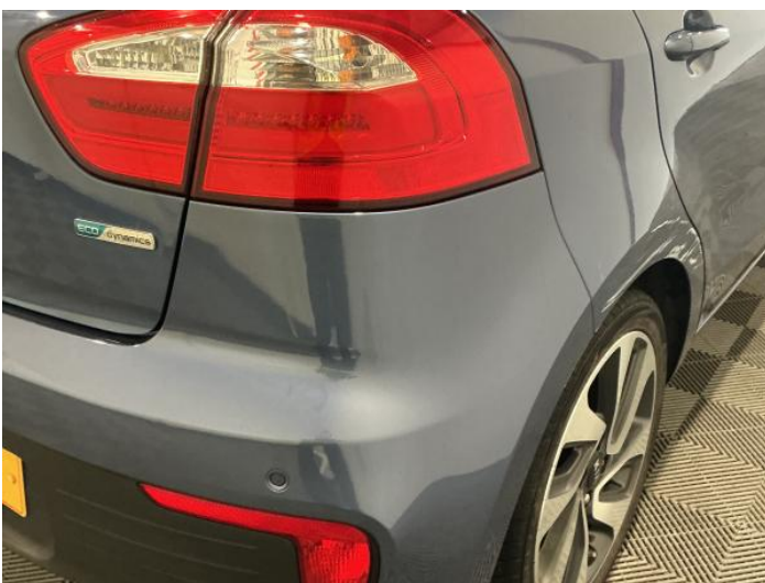
13: Bumper Rear Scratched 25 to 100mm Thru Paint
