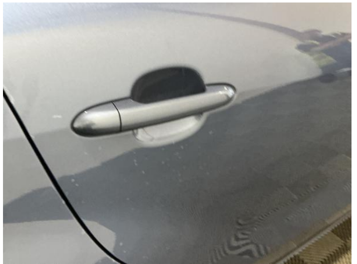
18: Door osr Chipped Multiple Chips
