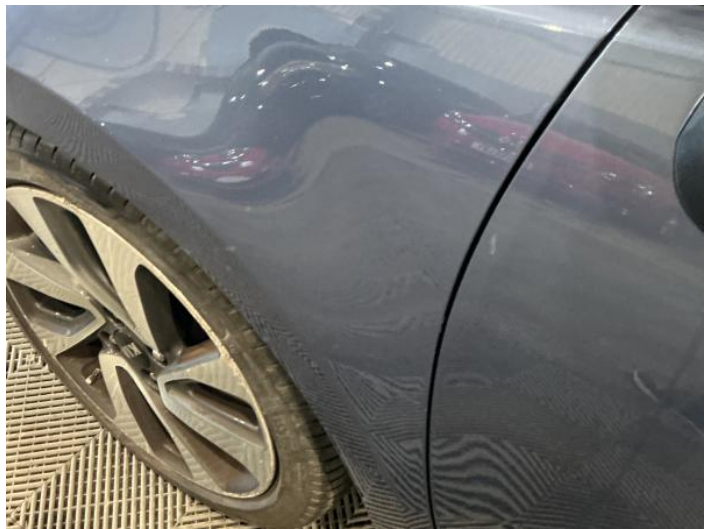
6: Wing nsf Dented With Paint Damage
