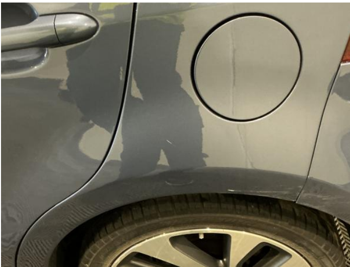
11: Qtr Panel nsr Dented With Paint Damage
