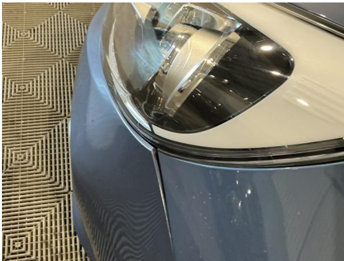
5: Bumper Front Insecure Action Required
