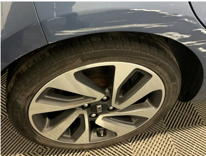
17: Wheel osr Scratched Up To 50mm
