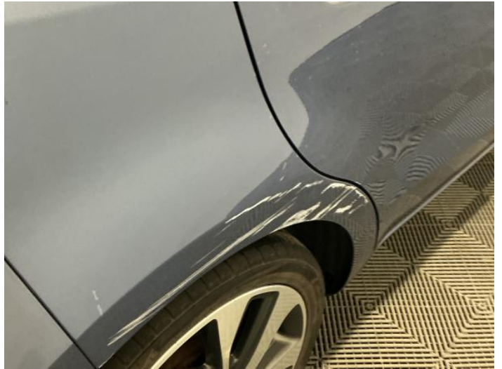
16: Qtr Panel osr Dented With Paint Damage
