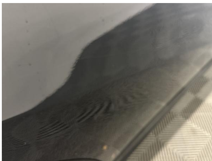
12: Door osr Scratched Over 25mm Thru Paint
