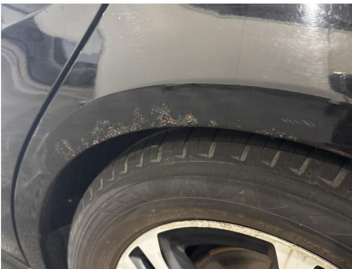
7: Qtr Panel nsr Rusted Over 5mm
