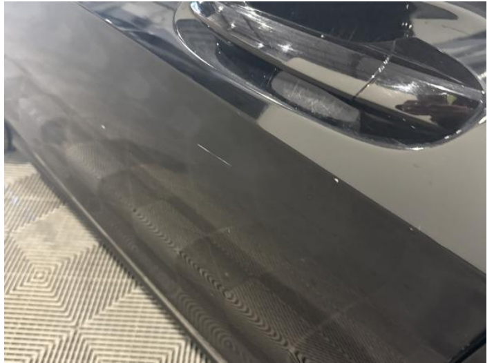
4: Door nsf Scratched Over 25mm Thru Paint
