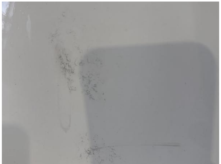
12: Qtr Panel nsr Poor Previous Repair Poor Paint
