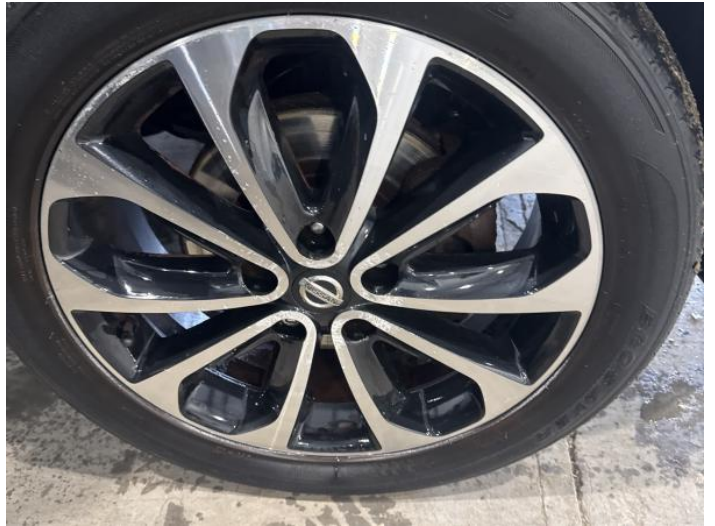
4: Wheel osf Scratched Over 50mm
