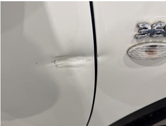
5: Door osf Dented With Paint Damage
