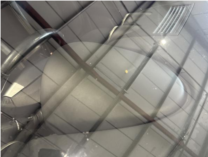
3: Screen Front Chipped UpTo 10mm
