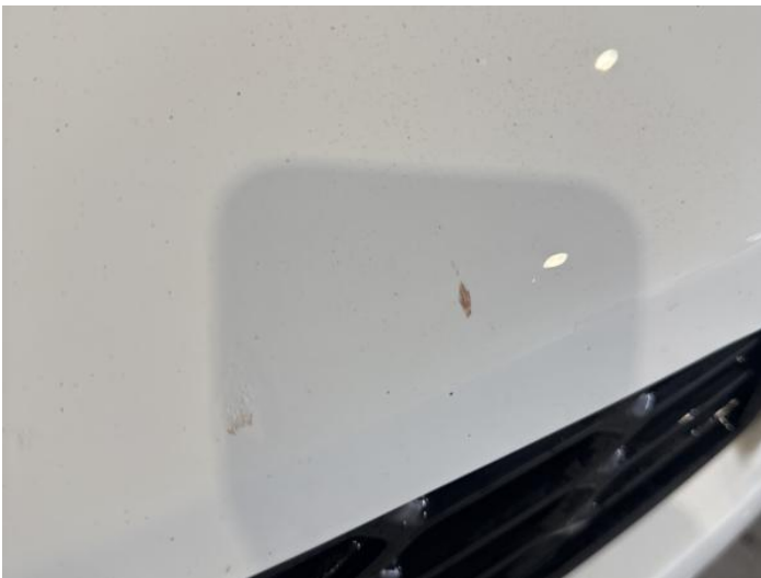
1: Bonnet Poor Previous Repair Poor Paint
