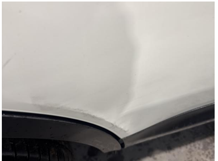
6: Door osr Dented With Paint Damage
