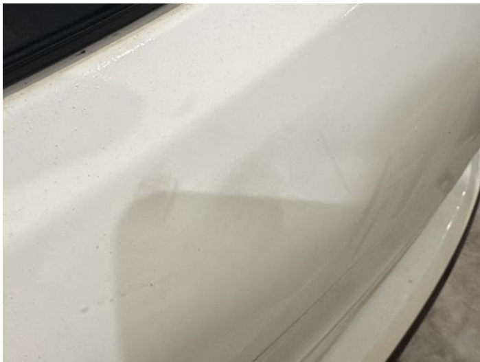
9: Boot Lid Poor Previous Repair Poor Paint
