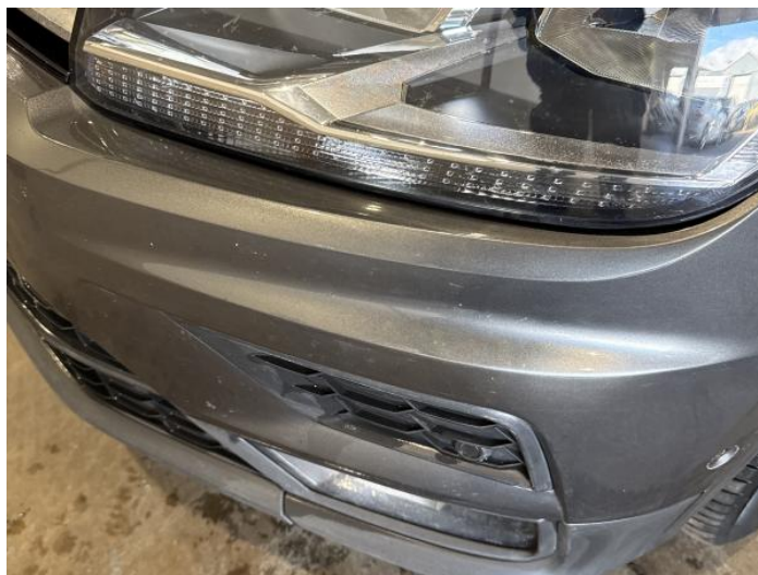
2: Bumper Front Scratched 25 to 100mm Thru Paint
