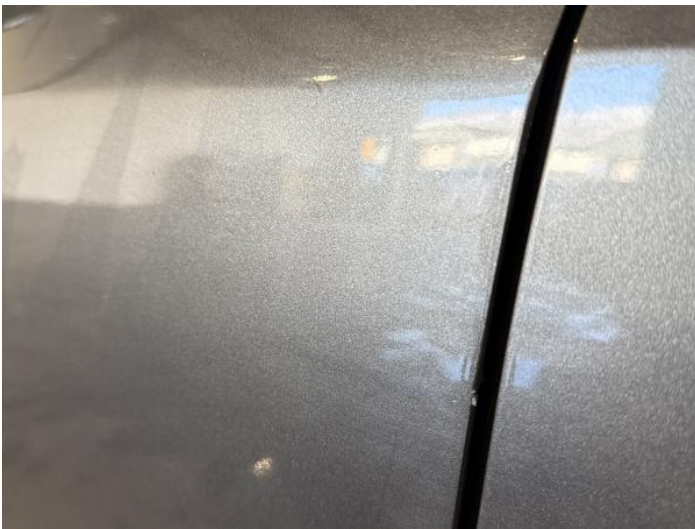
5: Door nsf Poor Previous Repair Poor Paint
