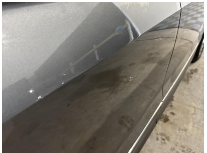
8: Door osr Dented 2 Or Less UpTo 10mm
