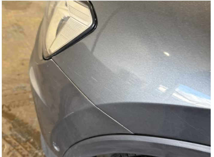
4: Wing nsf Scratched UpTo 25mm Thru Paint
