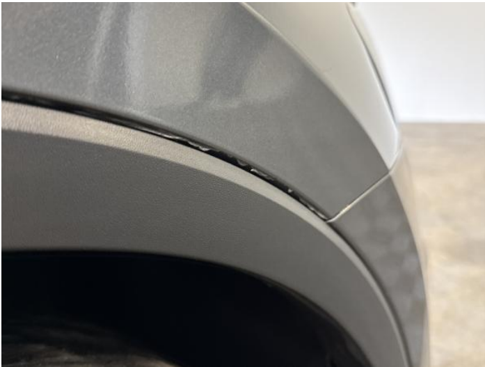
11: Wing osf Poor Previous Repair Rippled UpTo 30%
