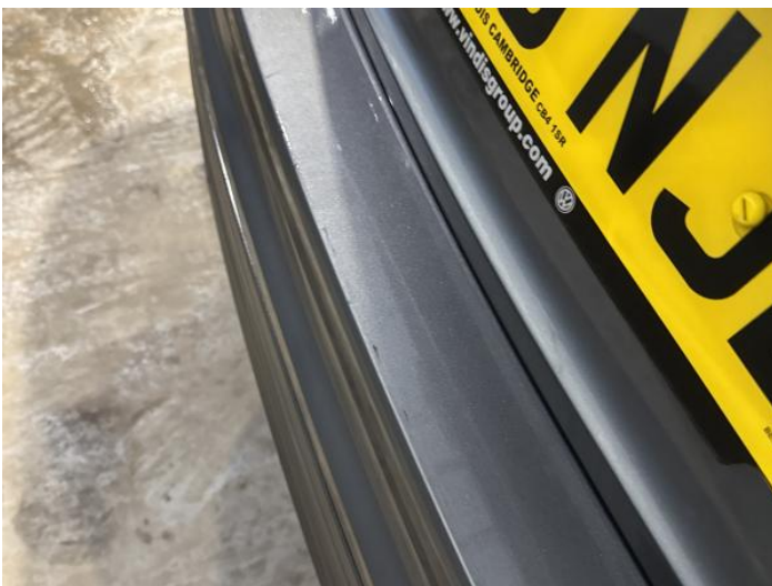
7: Bumper Rear Scratched 25 to 100mm Thru Paint
