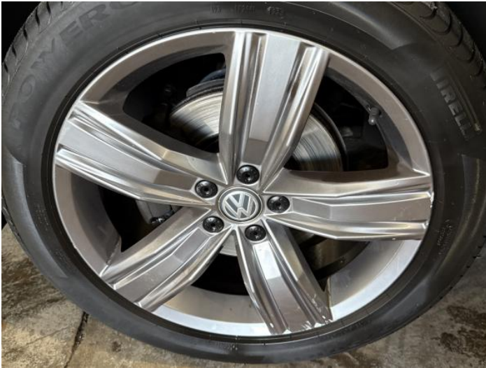
3: Wheel nsf Scratched Over 50mm
