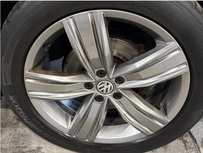
10: Wheel osf Scratched Up To 50mm
