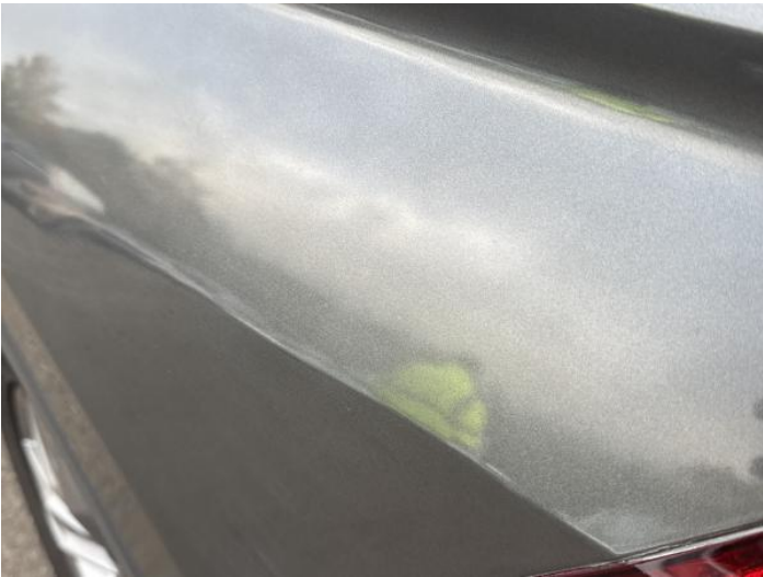
12: Qtr Panel nsr Poor Previous Repair Rippled UpTo 30%
