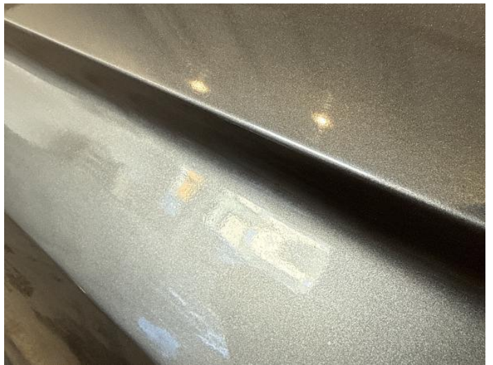
6: Door nsr Poor Previous Repair Poor Paint
