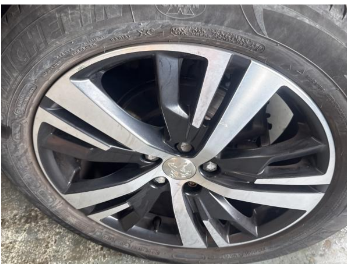
7: Wheel nsr Scratched Over 50mm
