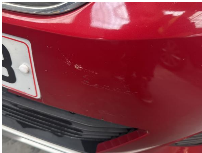
2: Bumper Front Scratched 25 to 100mm Thru Paint
