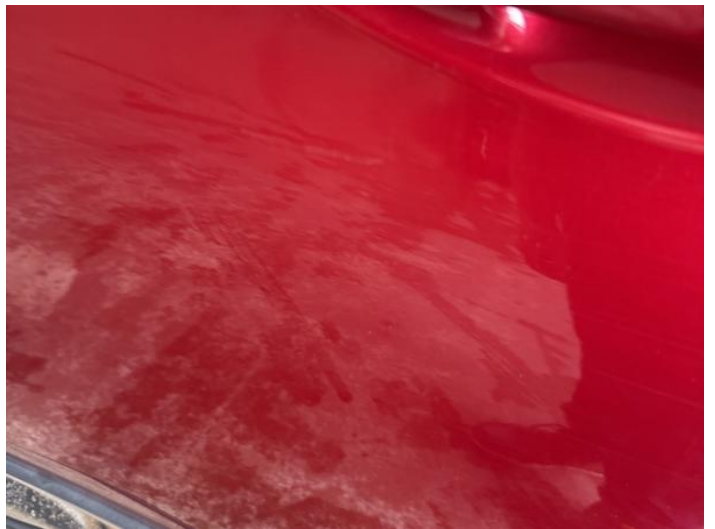
6: Door nsr Scratched Over 25mm Thru Paint
