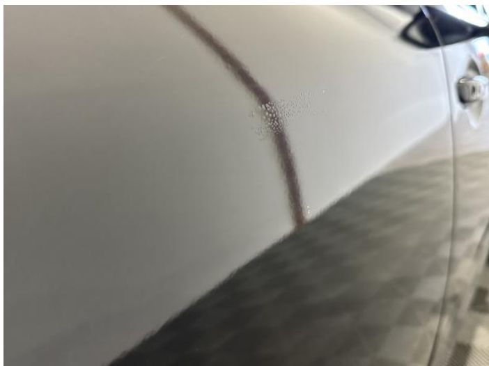
15: Door osr Poor Previous Repair Poor Paint
