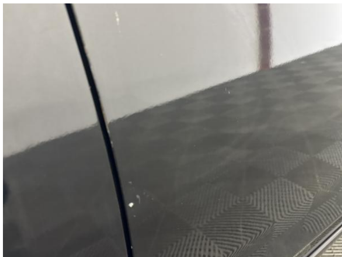
16: Door osf Scratched UpTo 25mm Thru Paint
