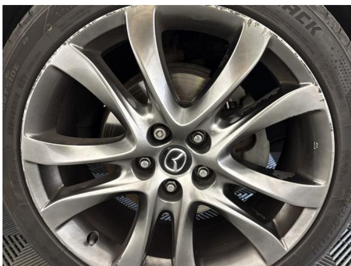
17: Wheel osf Scratched Over 50mm
