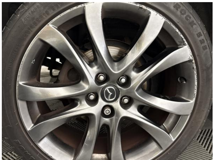
14: Wheel osr Scratched Over 50mm
