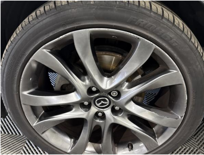
3: Wheel nsf Dented UpTo 30mm (Alloy)
