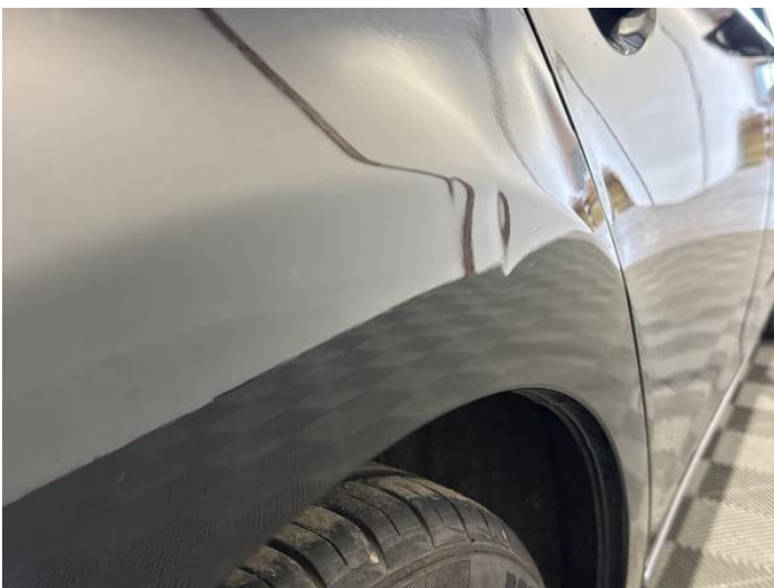
13: Qtr Panel osr Dented Over 30mm
