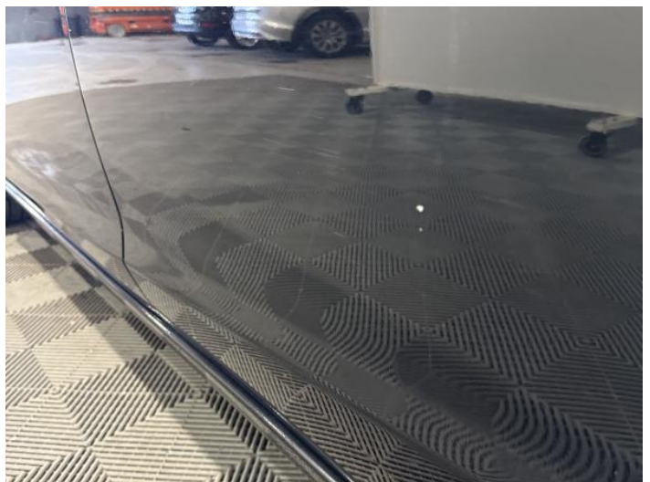
8: Door nsr Dented Between 10mm + 30mm
