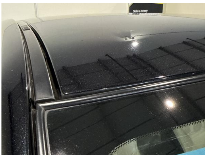
19: Roof Dented Over 30mm
