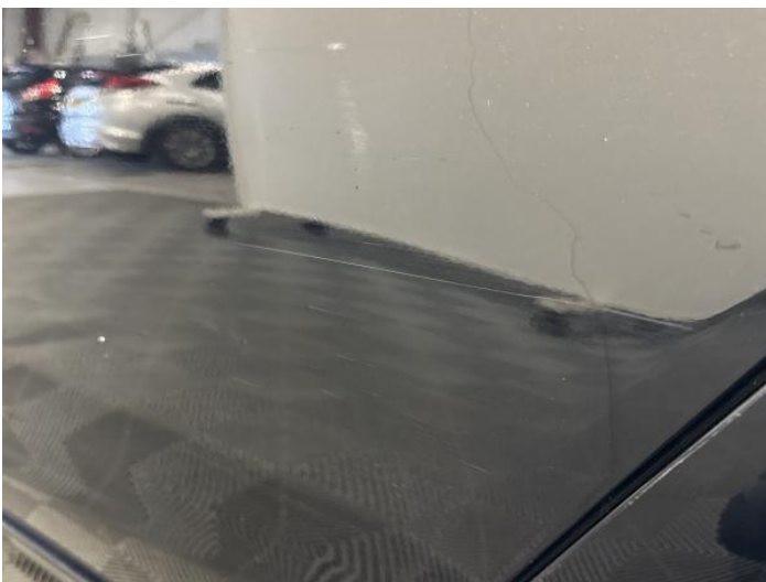
7: Door nsr Scratched Over 25mm Thru Paint
