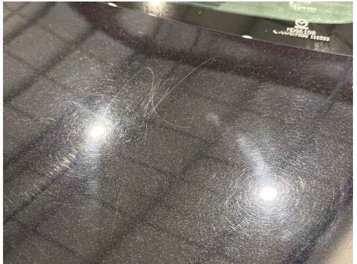
12: Boot Lid Scratched Over 25mm Thru Paint
