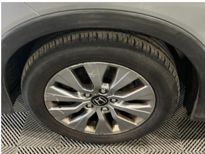
3: Wheel nsf Scratched Over 50mm
