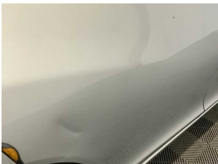
13: Door osr Dented Over 30mm
