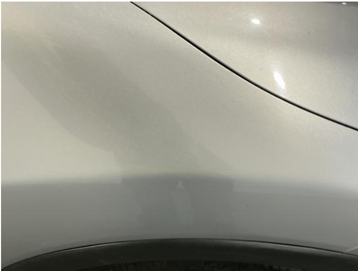
17: Wing osf Dented Over 2 UpTo 10mm
