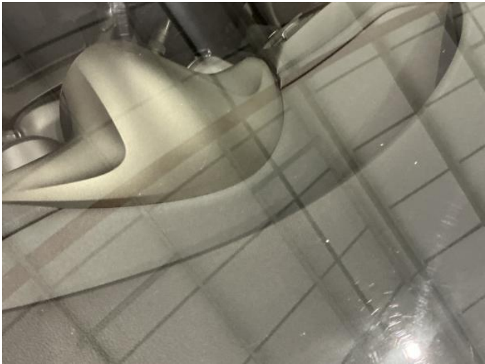
18: Screen Front Chipped UpTo 10mm
