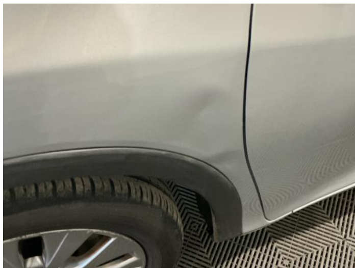
4: Wing nsf Dented Over 30mm
