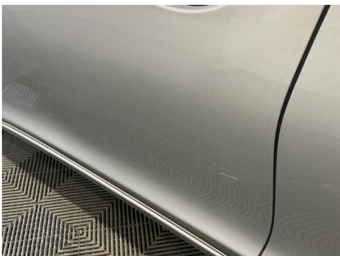
5: Door nsf Scratched Over 25mm Thru Paint
