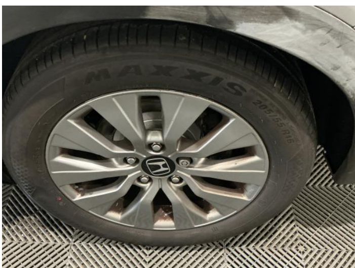
7: Wheel nsr Scratched Over 50mm
