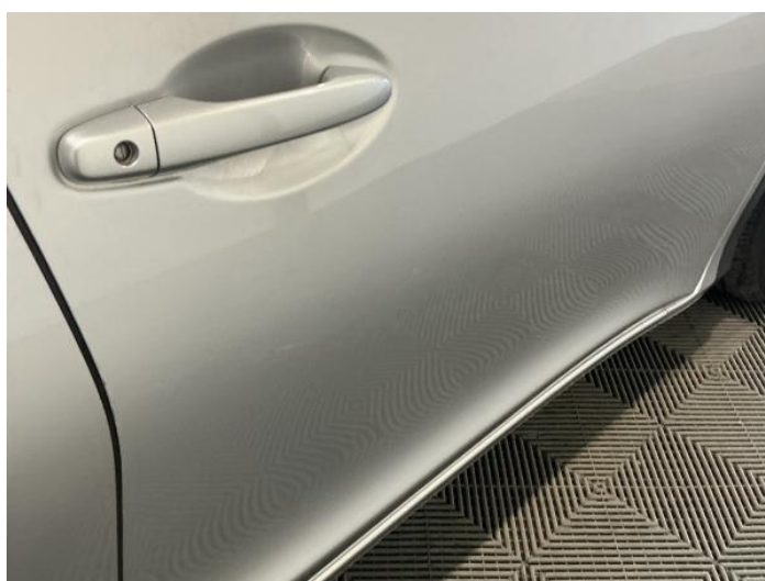
14: Door osf Dented With Paint Damage
