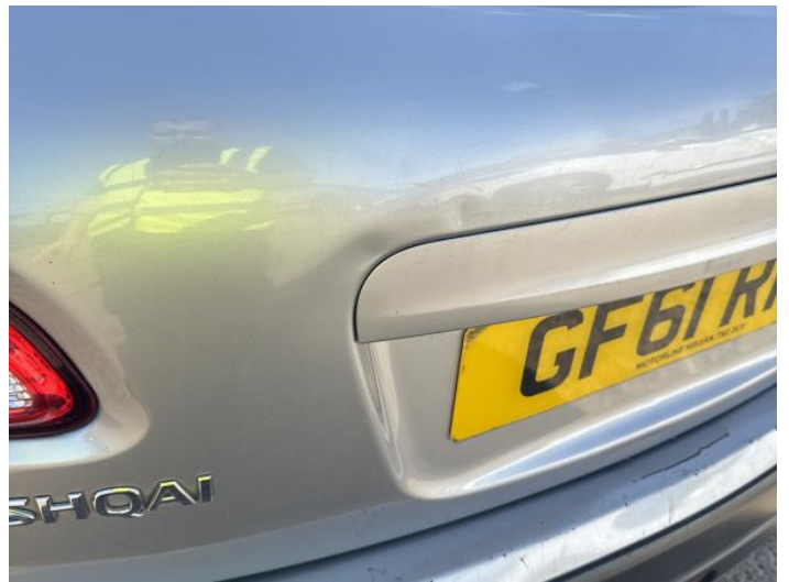
12: Boot Lid Dented Over 30mm
