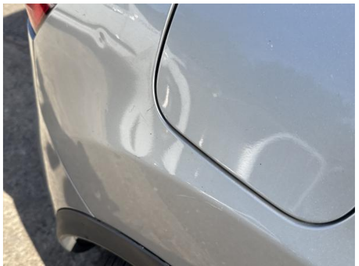
8: Qtr Panel osr Dented Between 10mm + 30mm
