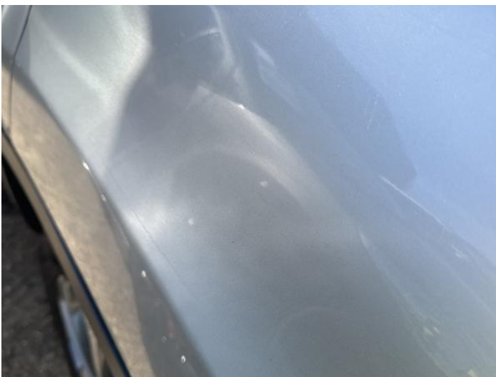
13: Qtr Panel nsr Chipped 1 To 5
