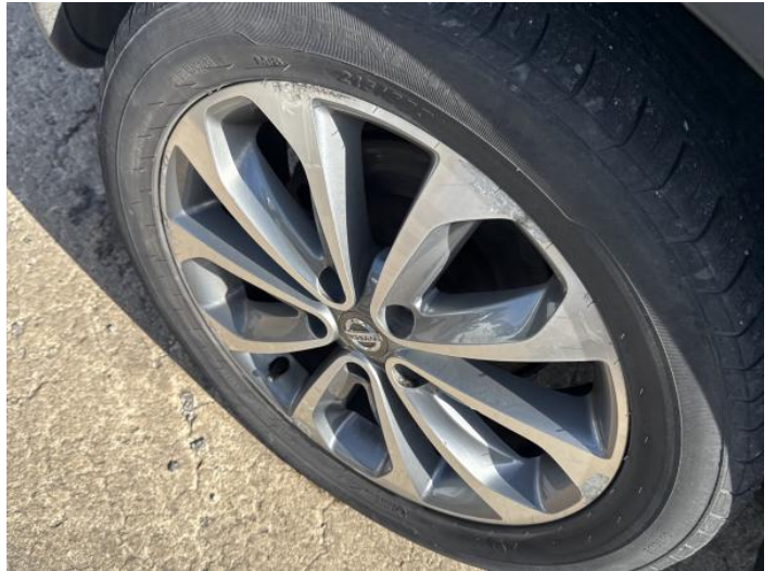
10: Wheel osr Scratched Over 50mm
