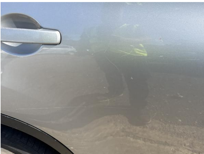
7: Door osr Dented With Paint Damage
