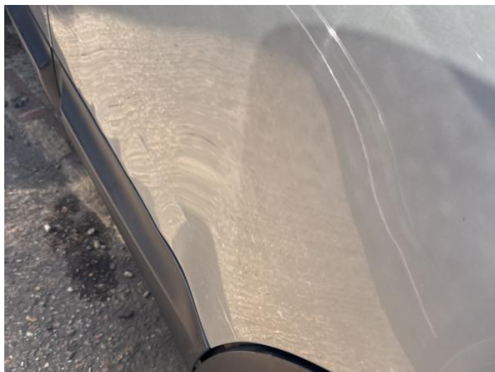
16: Door nsr Dented With Paint Damage
