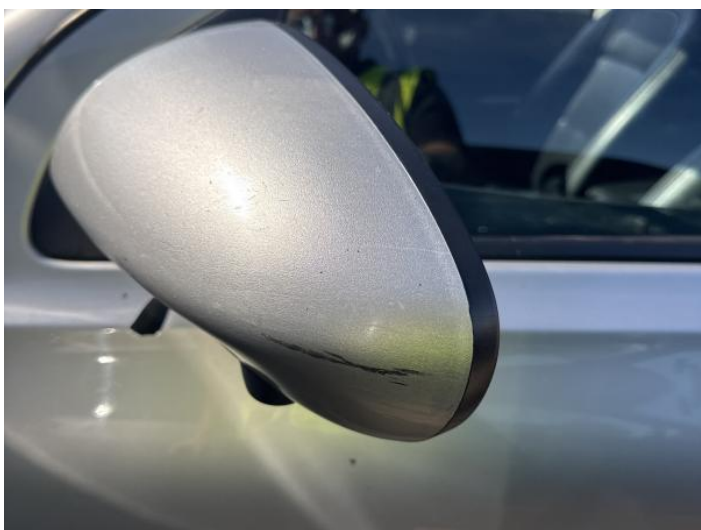
19: Door Mirror Assy nsf Scratched (Painted) Over 25mm Thru Paint
