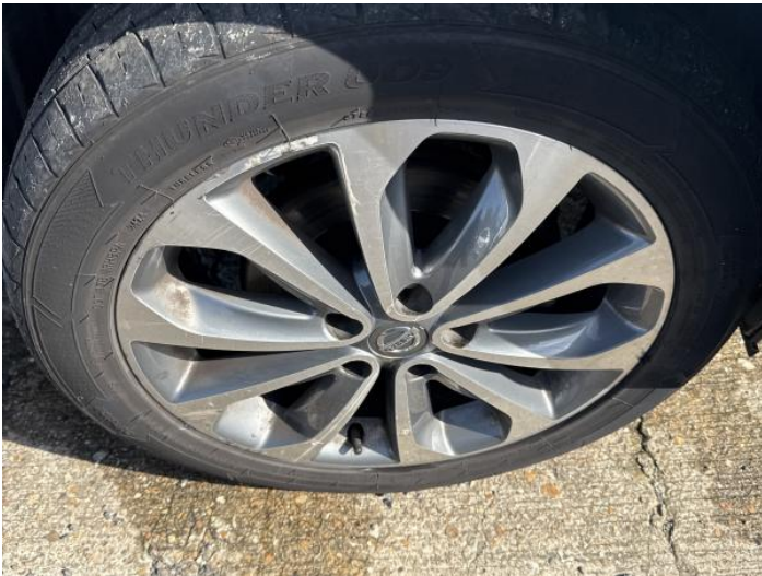
5: Wheel osf Scratched Over 50mm
