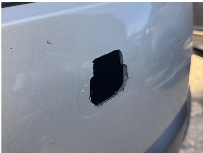
1: Bumper Front Hole Over 25mm
