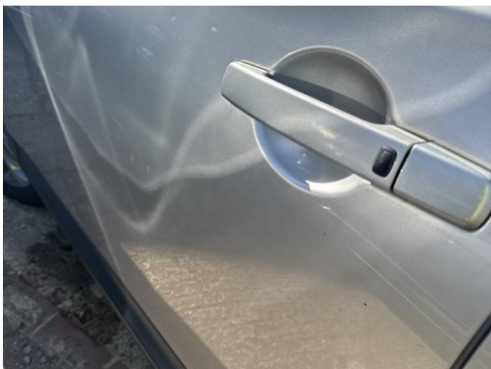
17: Door nsf Chipped 1 To 5
