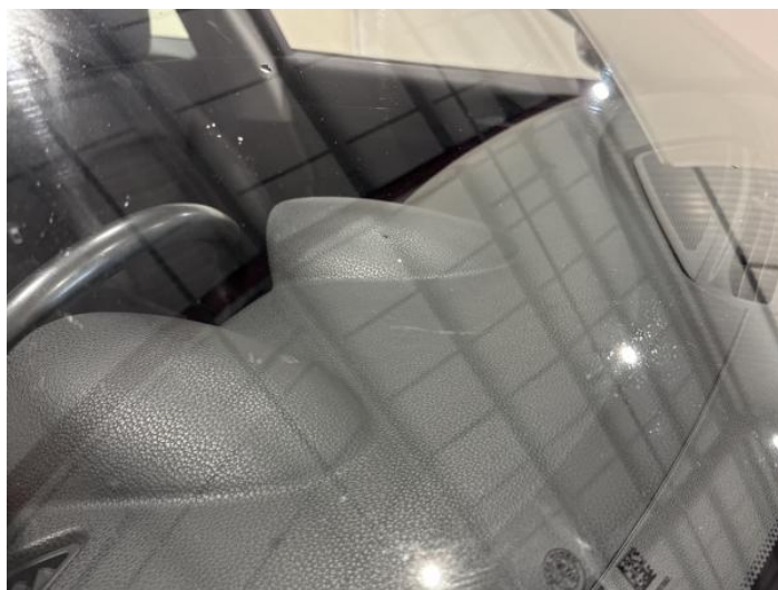
12: Screen Front Chipped UpTo 10mm
