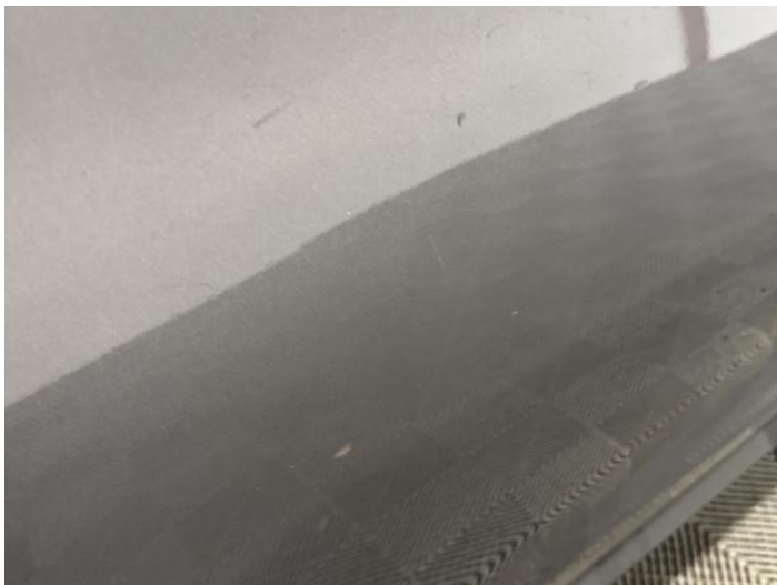
9: Door osr Scratched UpTo 25mm Thru Paint
