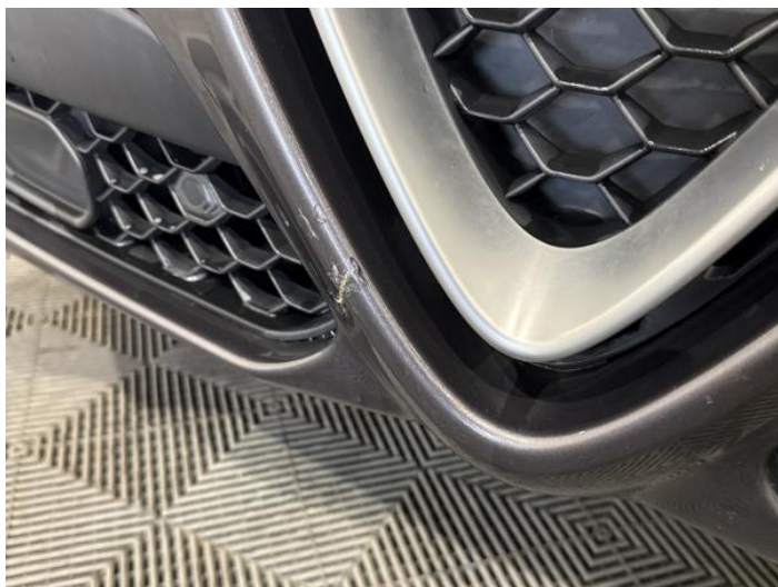
1: Bumper Front Cracked UpTo 25mm
