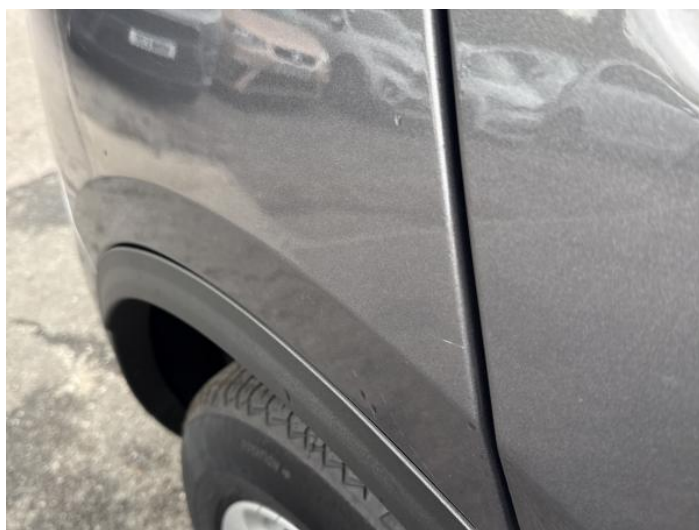
14: Qtr Panel osr Dented Over 30mm
