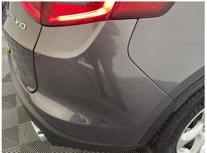
6: Bumper Rear Poor Previous Repair Poor Colour
