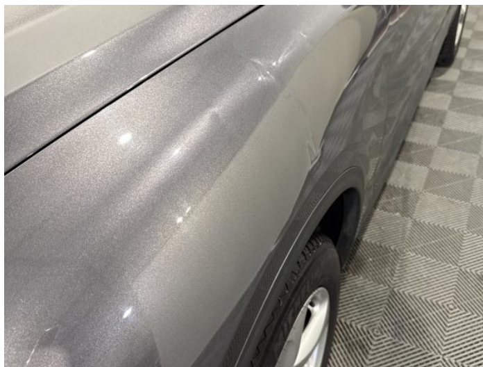
2: Wing nsf Dented Over 30mm
