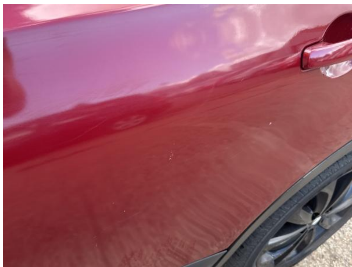
6: Door nsr Poor Previous Repair Poor Paint
