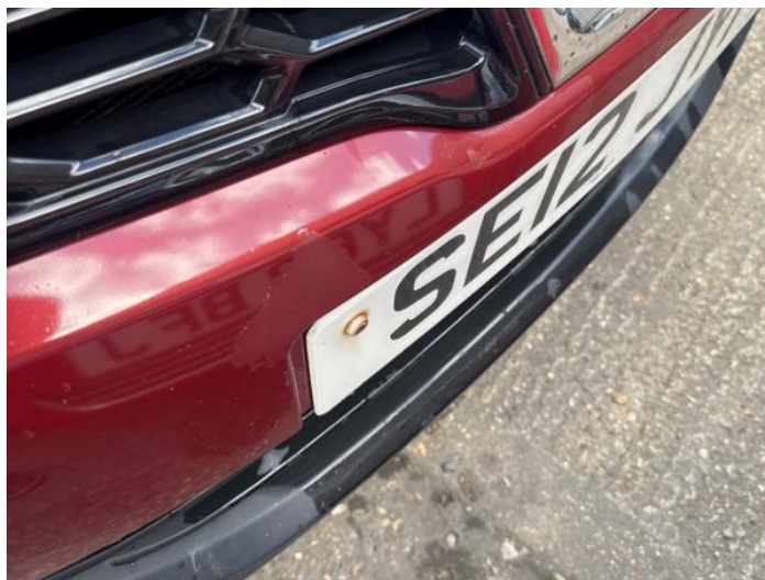
2: Bumper Front Poor Previous Repair Paint Flake
