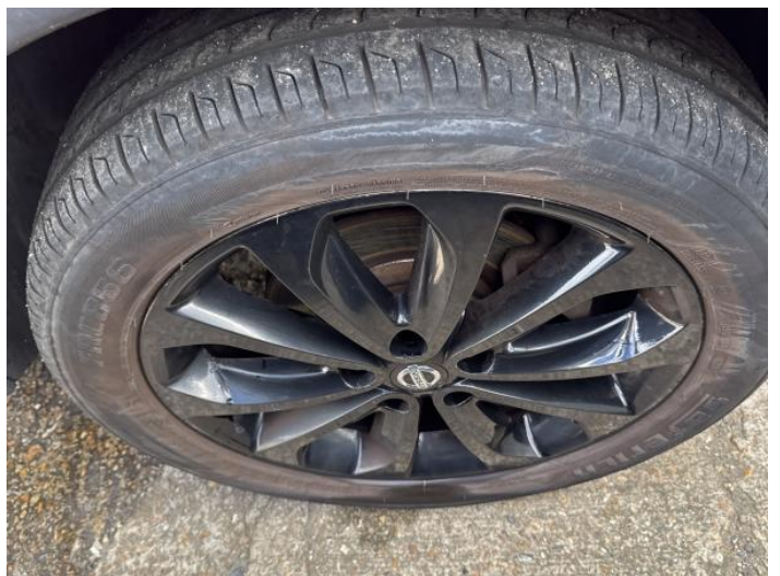
20: Wheel osf Scratched Over 50mm
