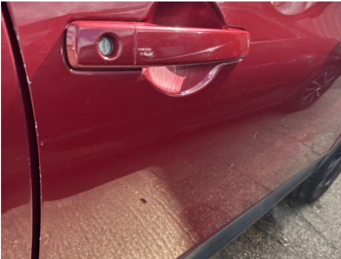
17: Door osf Dented With Paint Damage
