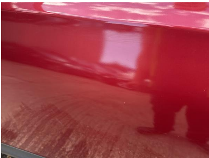
5: Door nsf Poor Previous Repair Poor Paint
