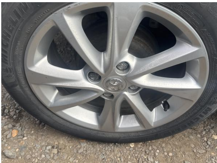
3: Wheel osr Scratched Up To 50mm
