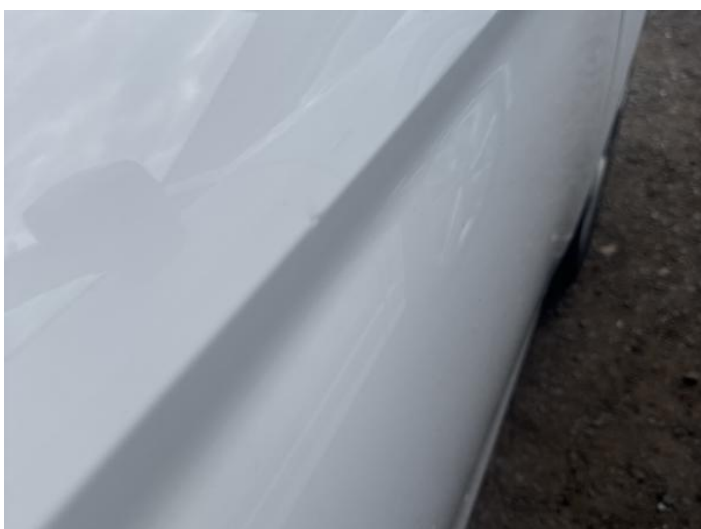
5: Door osf Dented Over 2 UpTo 10mm
