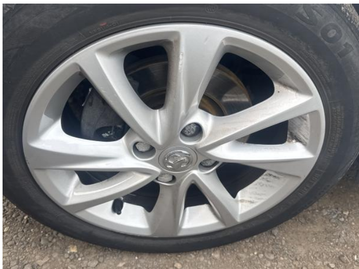
9: Wheel nsf Scratched Up To 50mm
