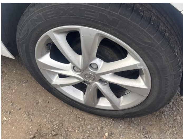
12: Wheel nsr Scratched Over 50mm
