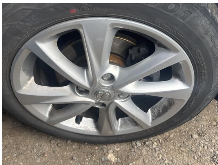
6: Wheel osf Scratched Up To 50mm
