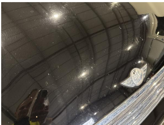
1: Bonnet Chipped Multiple Chips
