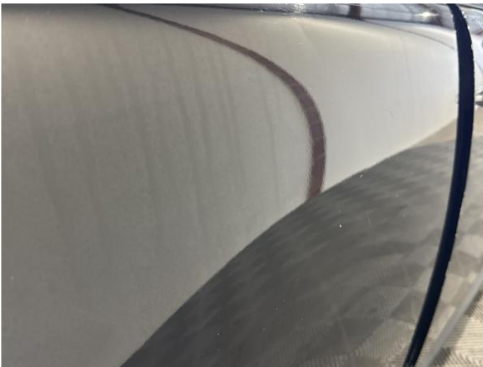
11: Qtr Panel osr Dented Over 30mm
