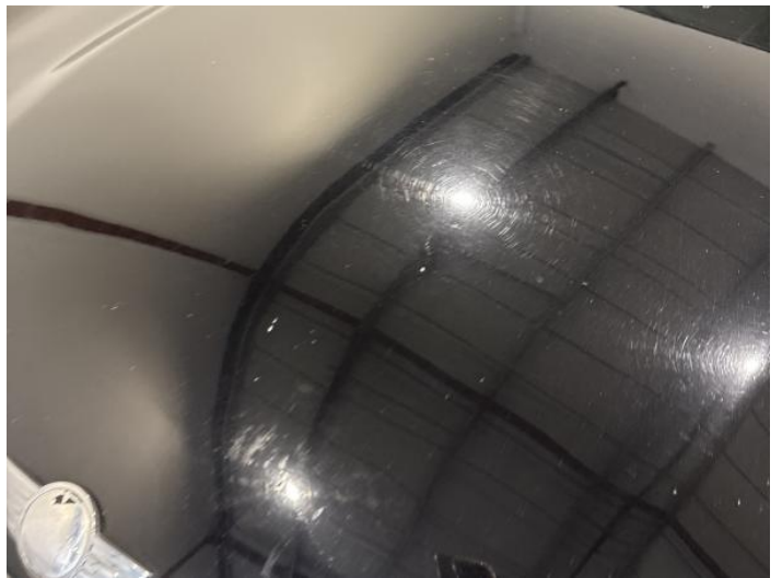
18: Bonnet Dented Between 10mm + 30mm
