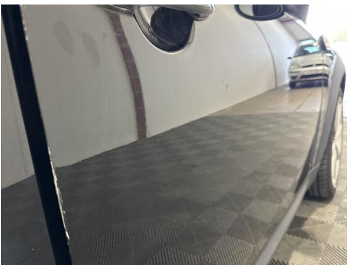
13: Door osf Poor Previous Repair Rippled UpTo 30%
