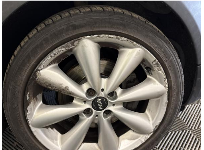
16: Wheel osf Scratched Over 50mm
