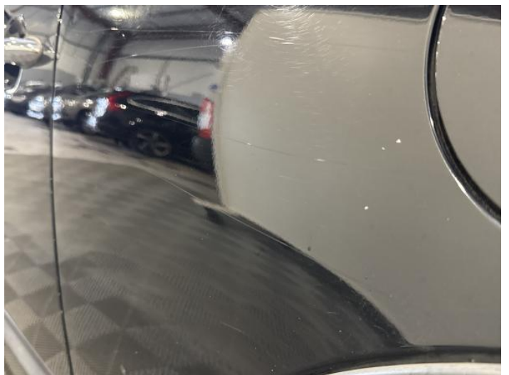
8: Qtr Panel nsr Chipped 1 To 5
