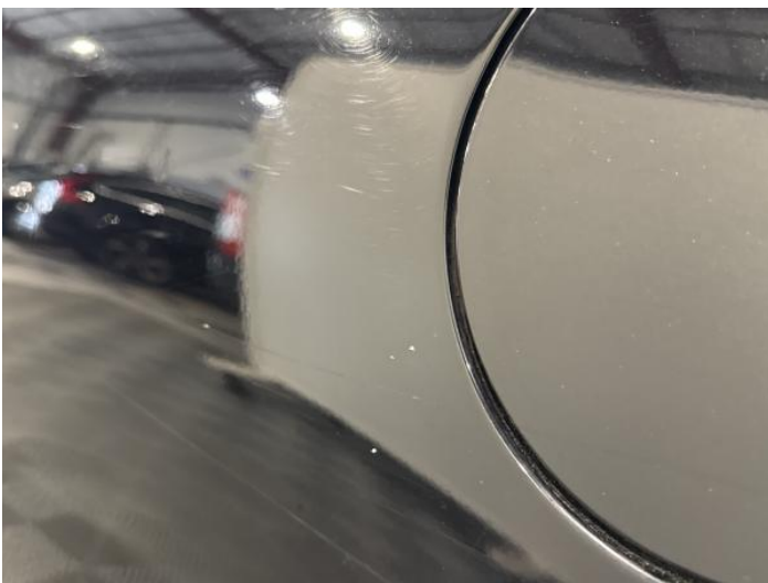
7: Qtr Panel nsr Dented Between 10mm + 30mm
