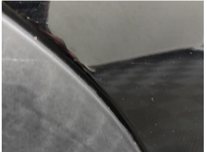
4: Wing nsf Scratched UpTo 25mm Thru Paint
