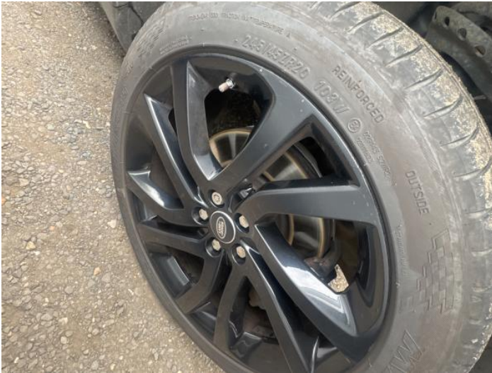
15: Wheel osf Scratched Up To 50mm
