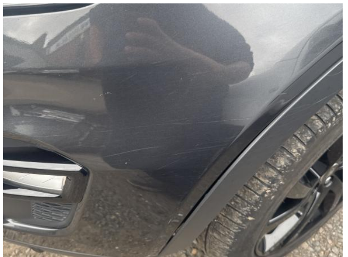
14: Bumper Front Scratched Over 100mm Thru Paint
