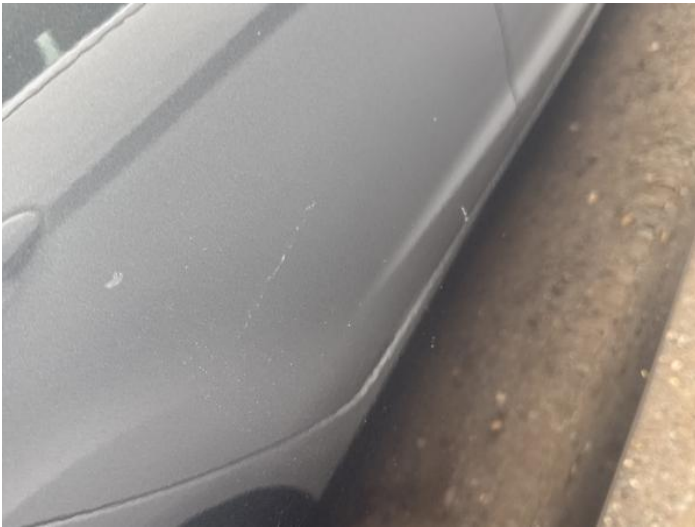
17: Door osf Chipped Multiple Chips
