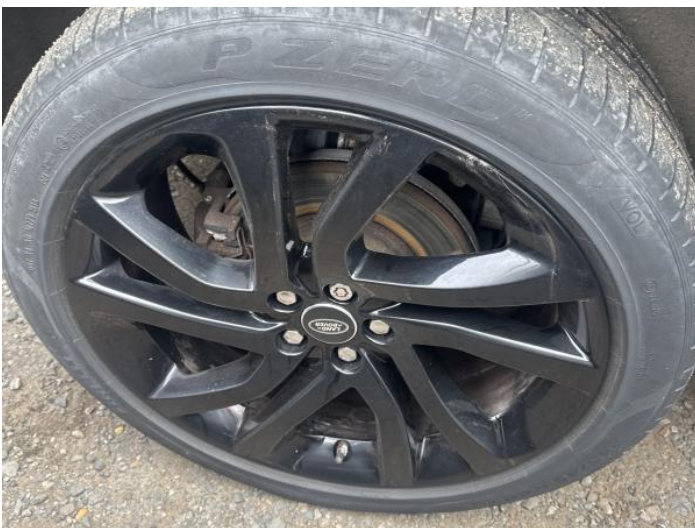
19: Wheel osr Scratched Up To 50mm
