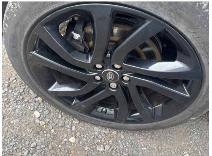
12: Wheel nsf Scratched Up To 50mm
