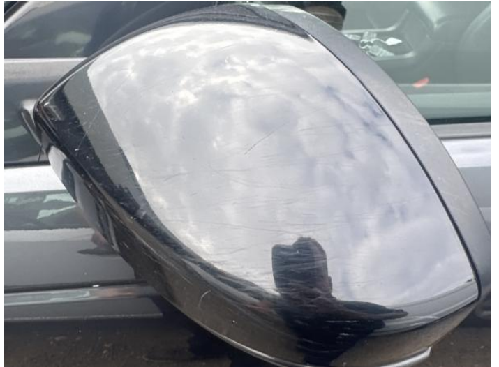
10: Door Mirror Assy nsf Scratched (Painted) Over 25mm Not Thru Paint
