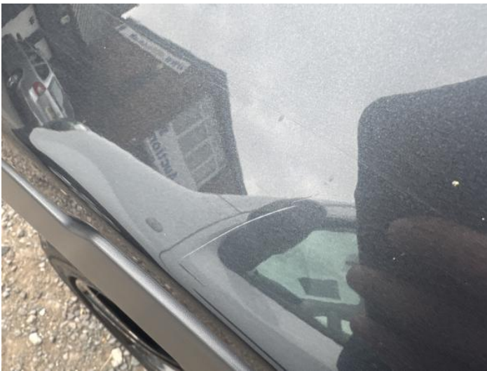
11: Wing nsf Scratched Over 25mm Thru Paint
