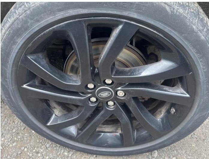
5: Wheel nsr Scratched Up To 50mm
