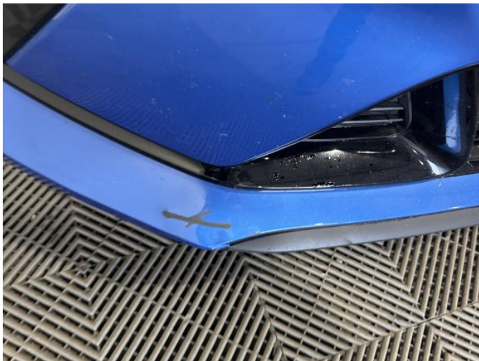
3: Bumper Front Cracked UpTo 25mm
