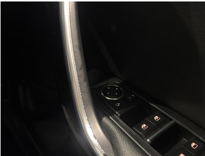
1: Handle Inner osf Damaged Replace
