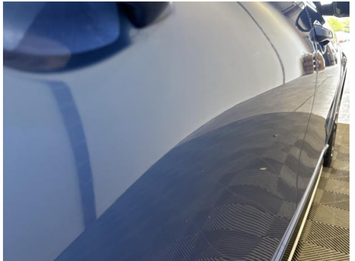
18: Door osr Dented Over 2 UpTo 10mm
