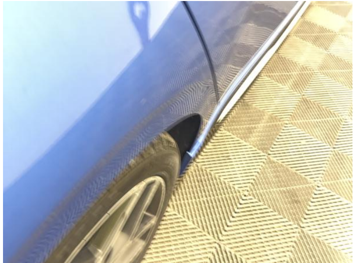
16: Qtr Panel osr Dented Over 30mm
