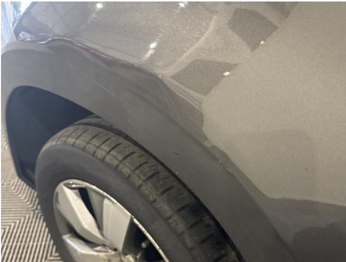
5: Wing nsf Dented Over 30mm
