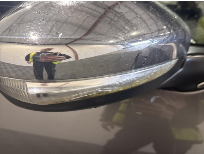
18: Flasher Side Repeater os Broken Replace
