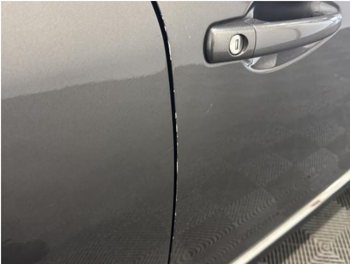
15: Door osf Chipped Edge Chip
