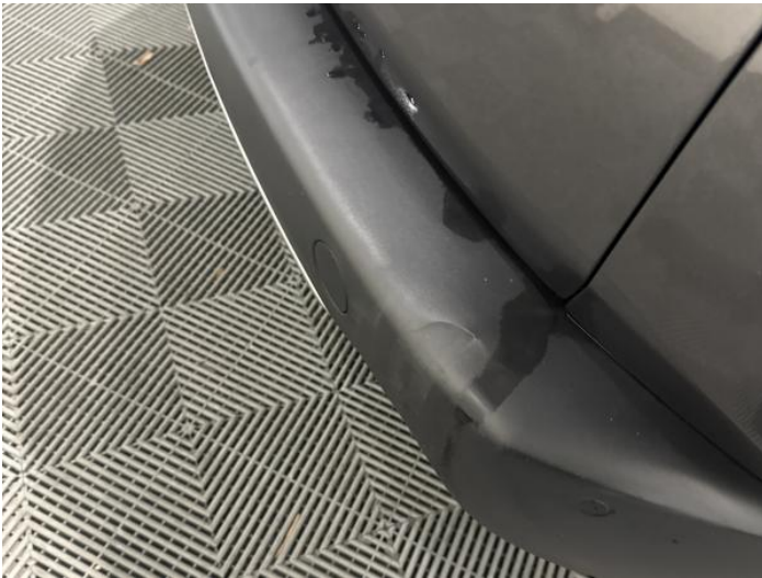
11: Bumper Rear Moulding Scuffed (Unpainted) UpTo 100mm
