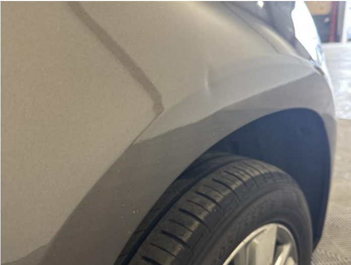
16: Wing osf Dented Between 10mm + 30mm
