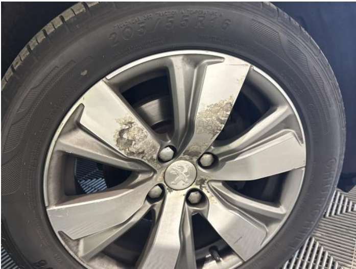
17: Wheel osf Scratched Over 50mm
