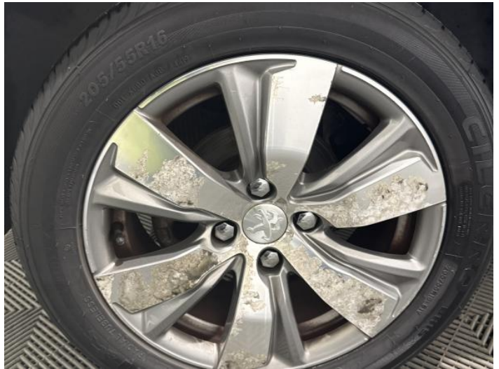
12: Wheel osr Scratched Over 50mm
