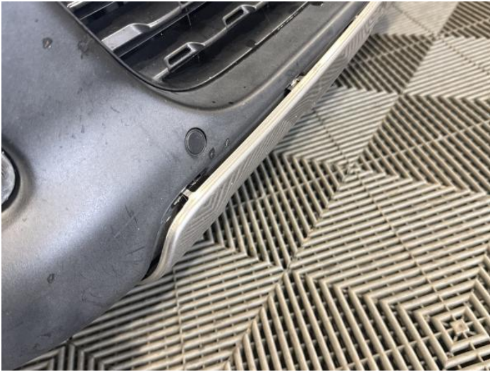
3: Bumper Front Moulding Broken Replace
