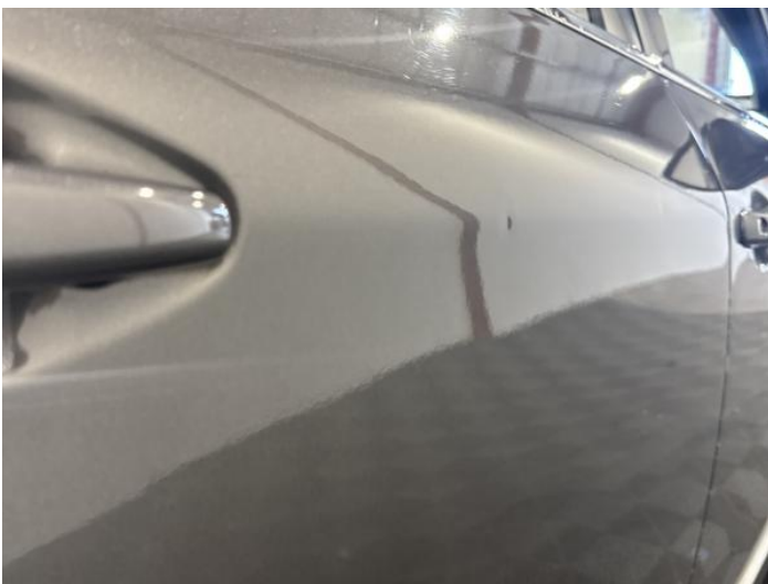
13: Door osr Dented Between 10mm + 30mm
