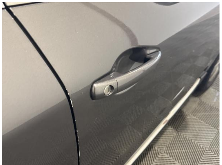
14: Door osf Dented Between 10mm + 30mm
