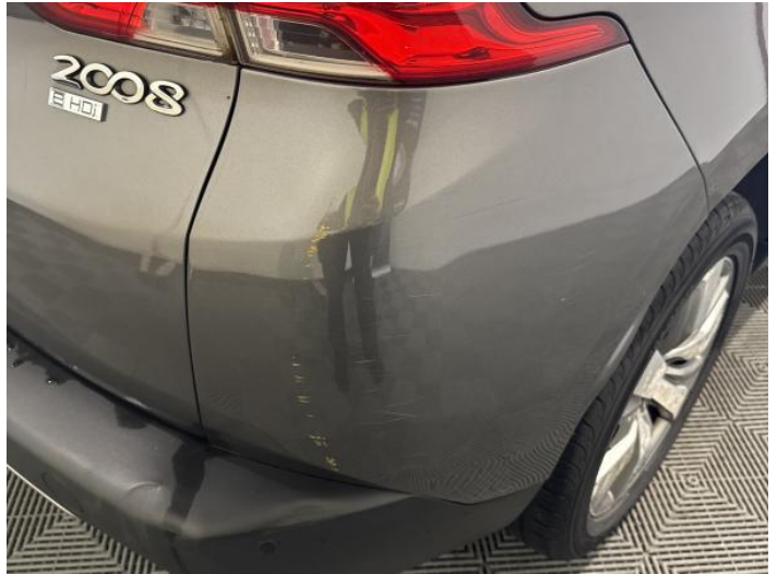
10: Bumper Rear Scratched Over 100mm Thru Paint
