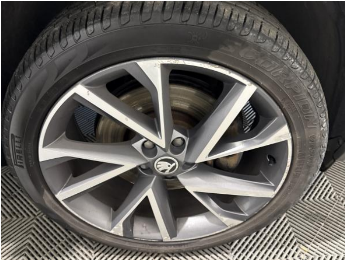
15: Wheel osf Scratched Over 50mm
