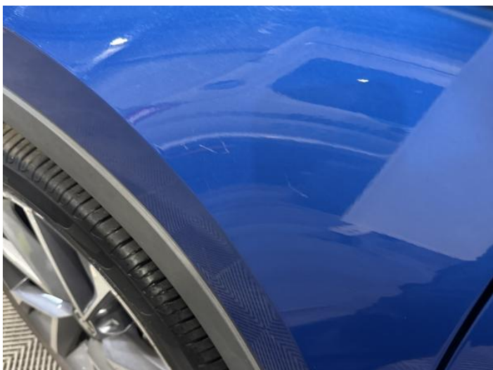
5: Wing nsf Scratched UpTo 25mm Thru Paint
