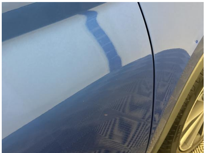
14: Door osf Dented Between 10mm + 30mm
