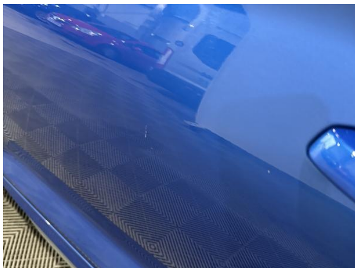
6: Door nsf Scratched UpTo 25mm Thru Paint
