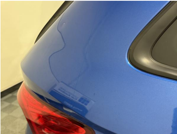
17: Qtr Panel osr Dented Between 10mm + 30mm
