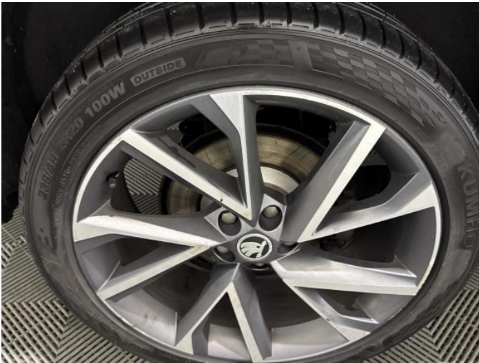
11: Wheel nsr Scratched Over 50mm
