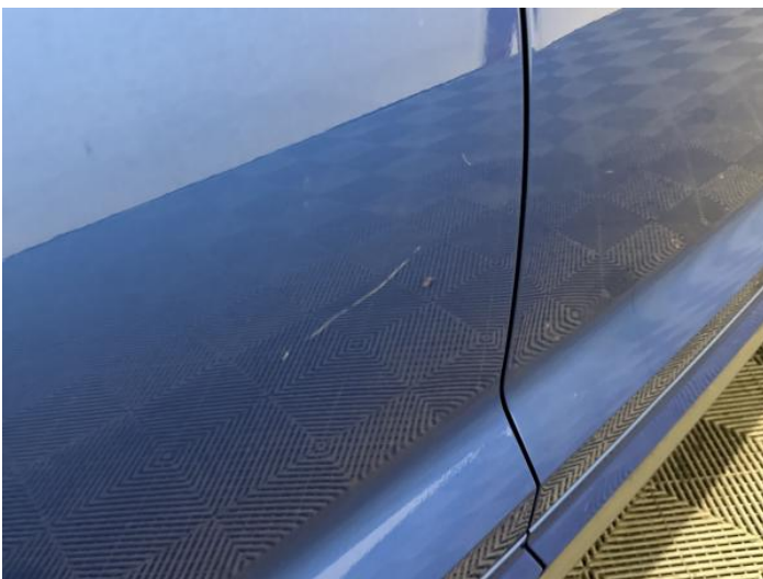
13: Door osr Scratched Over 25mm Thru Paint
