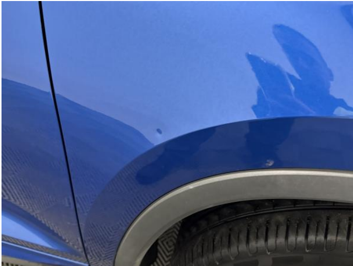
16: Wing osf Dented Between 10mm + 30mm
