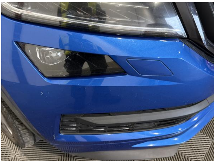
3: Bumper Front Chipped Multiple Chips
