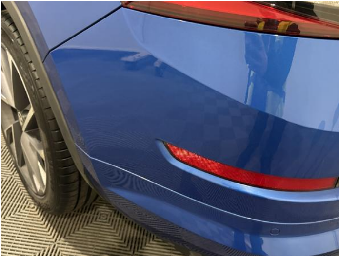
9: Bumper Rear Scratched 25 to 100mm Thru Paint
