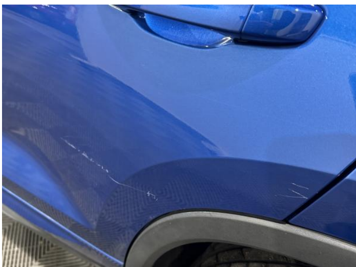
7: Door nsr Scratched Over 25mm Thru Paint
