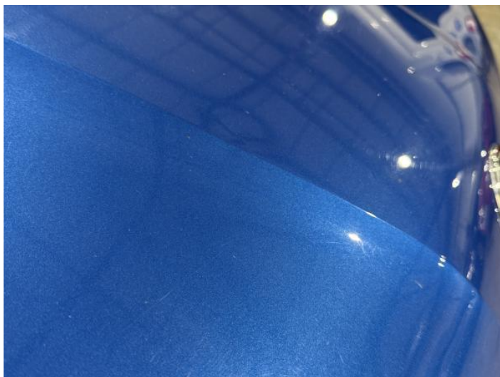
1: Bonnet Dented Between 10mm + 30mm
