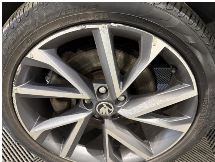
4: Wheel nsf Scratched Over 50mm
