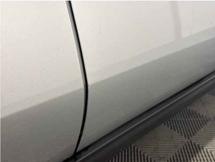
10: Door osf Chipped Edge Chip
