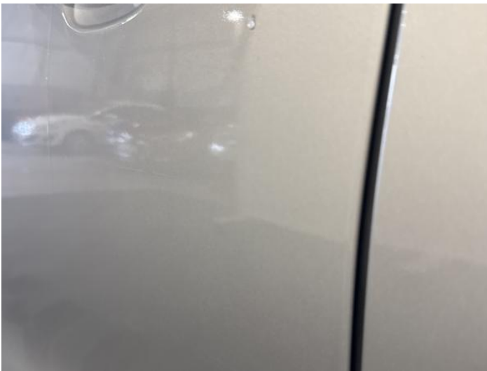
5: Door nsf Scratched Up To 25mm Thru Paint
