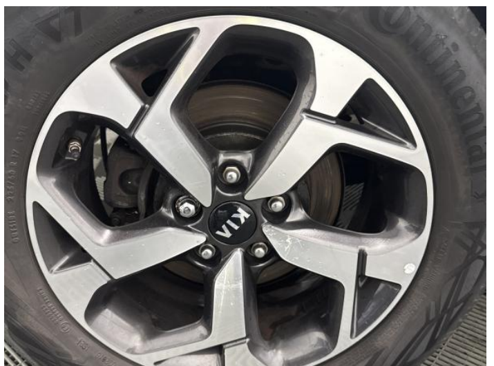
8: Wheel osr Scratched Over 50mm
