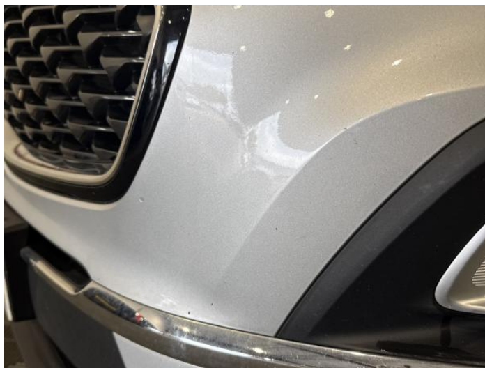
2: Bumper Front Chipped Multiple Chips
