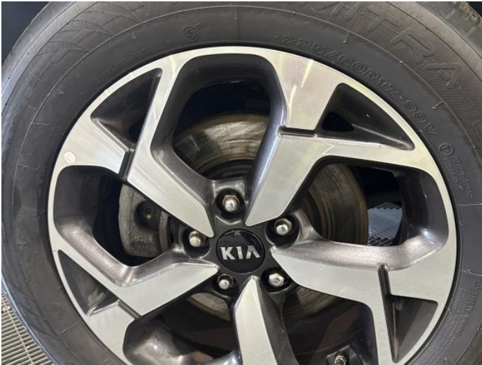
3: Wheel nsf Scratched Up To 50mm
