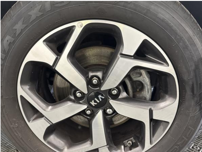
11: Wheel osf Scratched Up To 50mm
