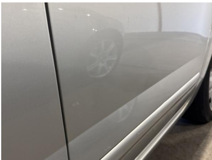
11: Door nsr Dented Over 30mm
