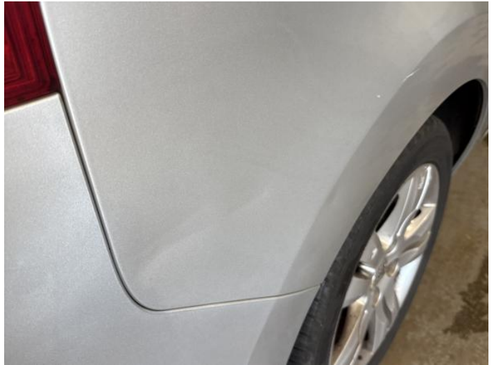
16: Qtr Panel osr Dented Over 30mm
