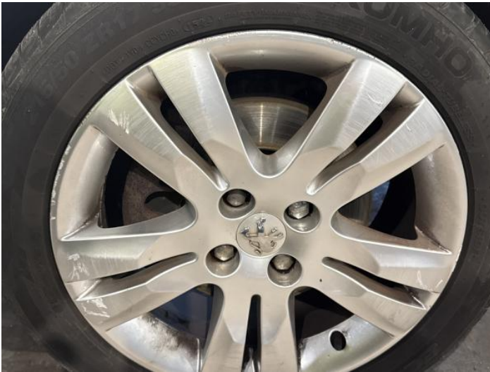
5: Wheel nsf Scratched Over 50mm
