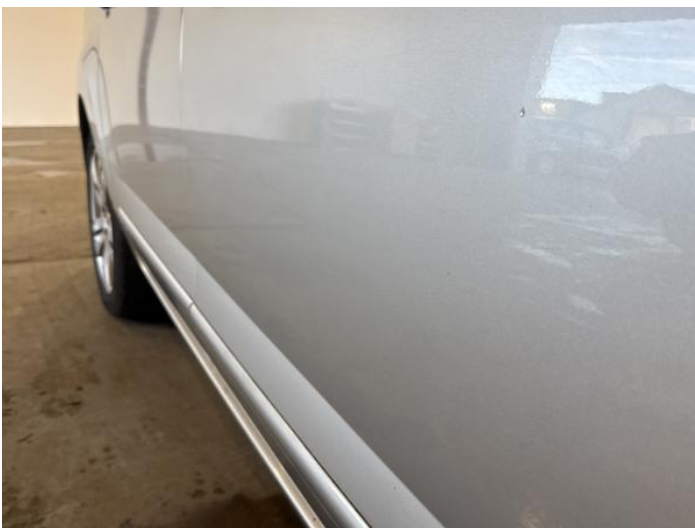
19: Door osf Dented Between 10mm + 30mm
