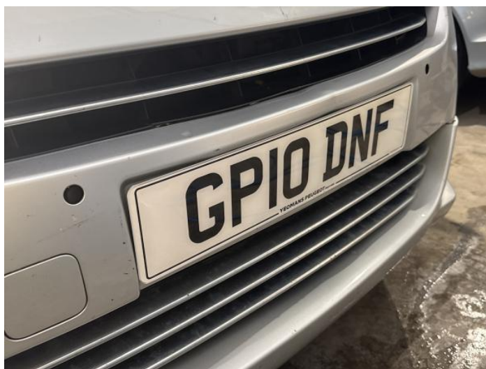
2: Parking Sensor Front Missing Replace
