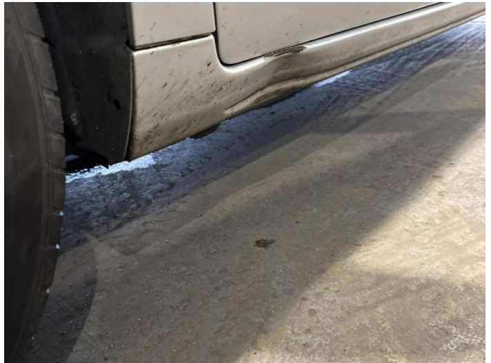
6: Sill ns Dented Over 30mm
