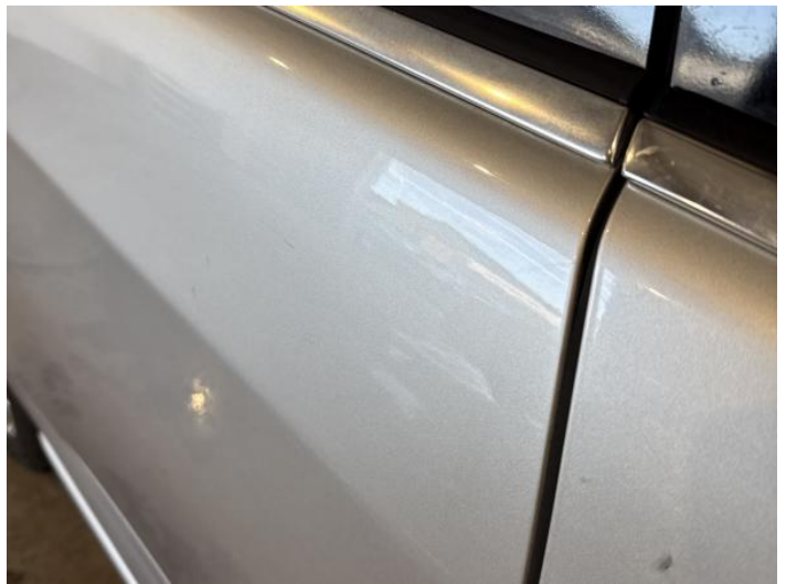
18: Door osr Scratched UpTo 25mm Thru Paint
