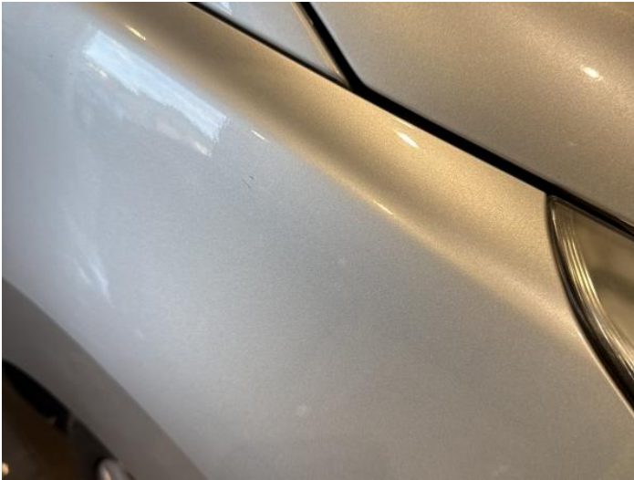
21: Wing osf Scratched UpTo 25mm Thru Paint
