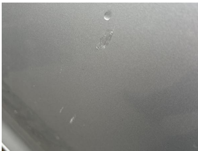
2: Door osf Scratched UpTo 25mm Thru Paint
