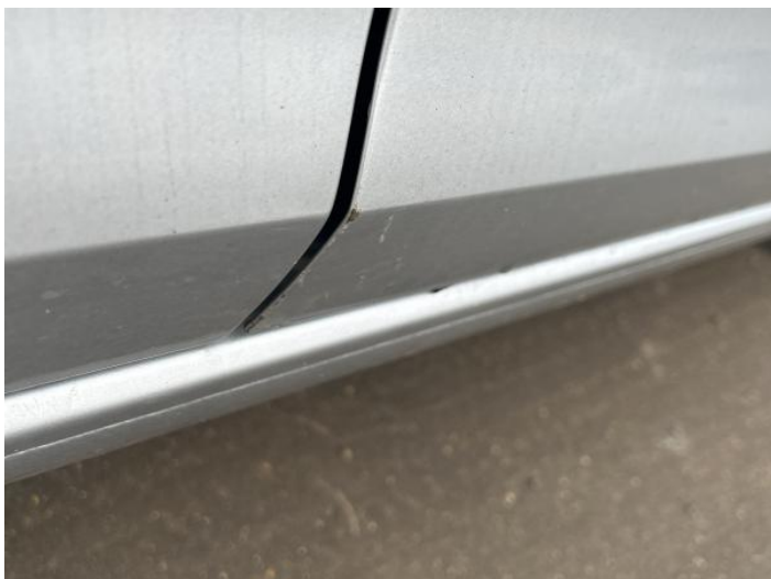
3: Door osf Chipped Edge Chip
