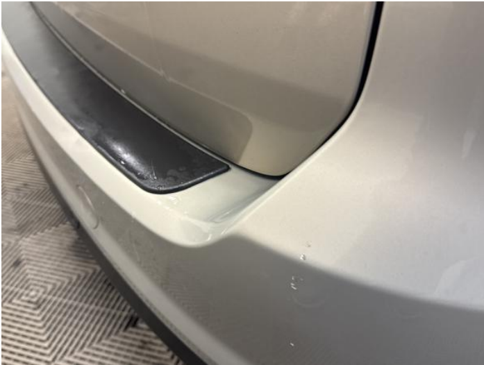
9: Bumper Rear Scratched Over 100mm Thru Paint
