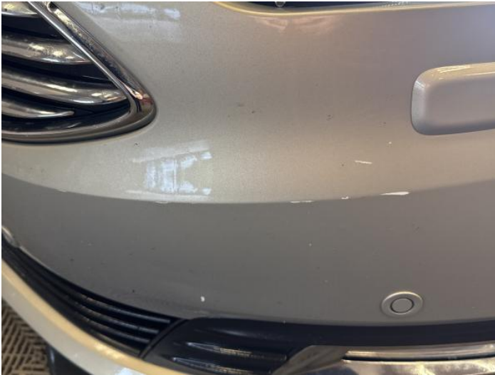
3: Bumper Front Scratched 25 to 100mm Thru Paint
