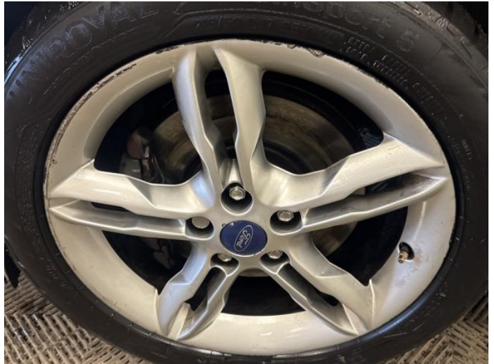
4: Wheel nsf Scratched Over 50mm
