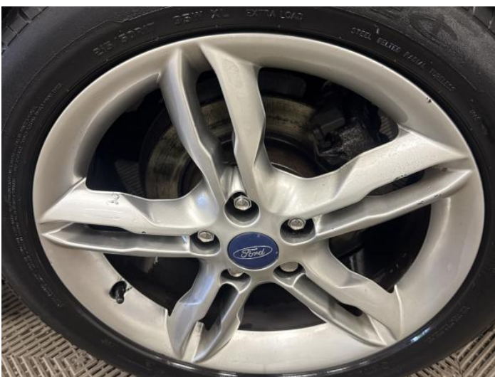
7: Wheel nsr Corroded Light
