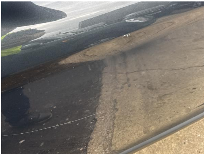
5: Door nsf Dented With Paint Damage
