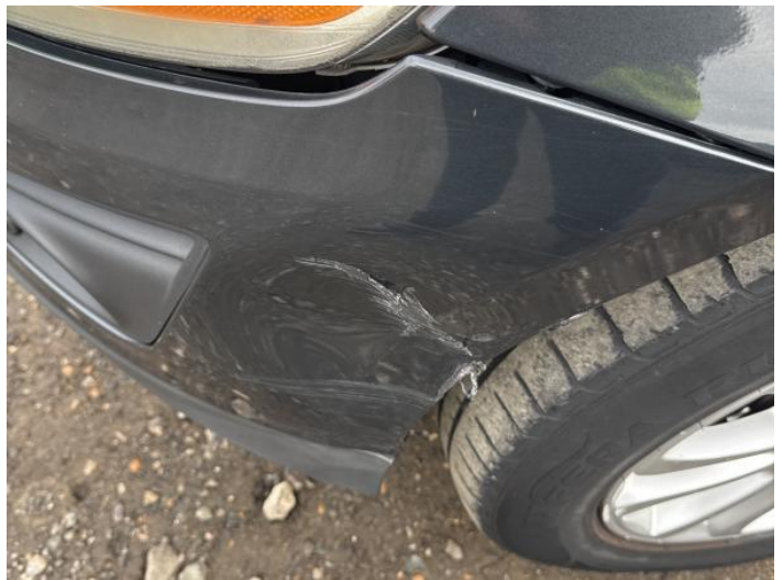
4: Bumper Front Cracked UpTo 25mm
