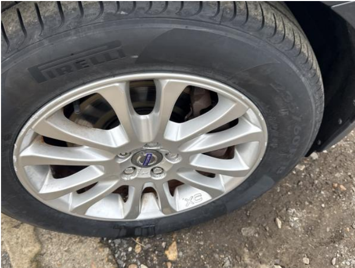
21: Wheel osf Scratched Over 50mm
